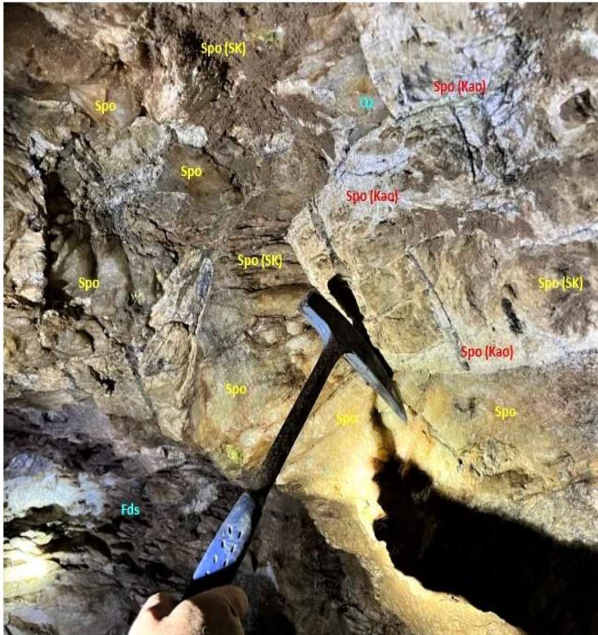
Figure 6: Typical of spodumene crystals within Spodumene Zone in Jaime Linopolis Sitio do Estevinho underground mine. Massive fresh spodumene (Spo) . White domains are partially kaolinized spodumene along fractures (Spo Kao). Spodumene with skeletal/corroded texture (Spo SK). Spodumene occupies at least 60% of the field of view in this picture.
