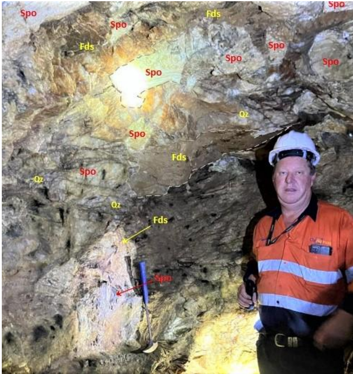
Figure 5: Coarse spodumene crystals (Spo) within Spodumene Zone in Jaime Linopolis Sitio do Estevinho underground mine. Other minerals are Feldspar (Fds) and Quartz (Qz) and black Tourmaline. Spodumene occupies at least 25 % of the field of view in this picture.
