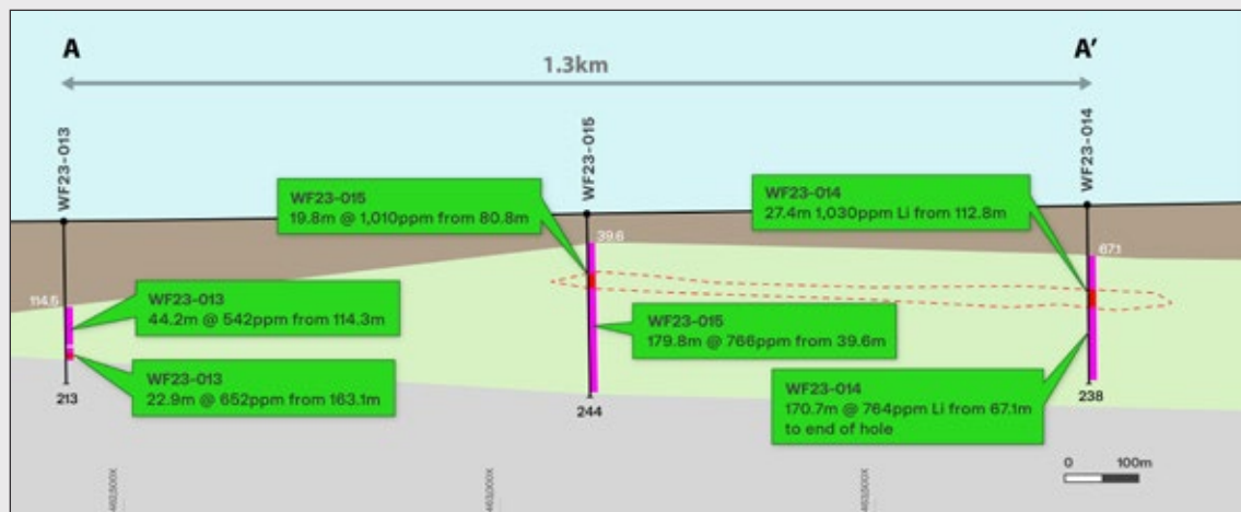
FIGURE 08 Schematic Cross Section 4218530N- RC drill hole's WF23-013-WF23-015
