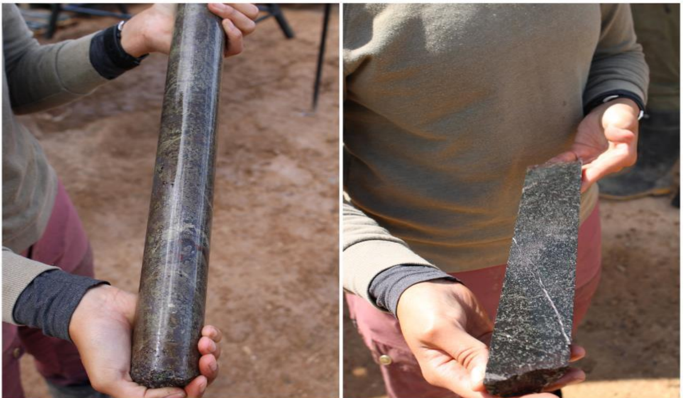
Figure 1: W56 prospect –WL23-367: 21.9m @ 1.02% Ni from 206.65m including 1.35m @ 5.02% Ni from 227.2m and 4.4m @ 1.55% Ni from 247.1m. Massive Sulphides at 227.2m and net texture sulphides at 248.5m, refer ASX on 11 July 2023.
