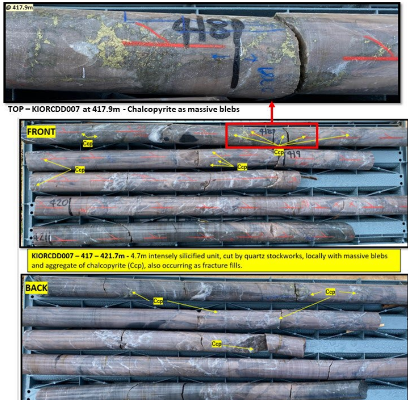
Figure 12: Drill hole KIORCDD007 – Intensely silicified meta sediment cut by quartz stockwork veins containing chalcopyrite as fracture fill and blebs (ASX: 6 July 2023).
