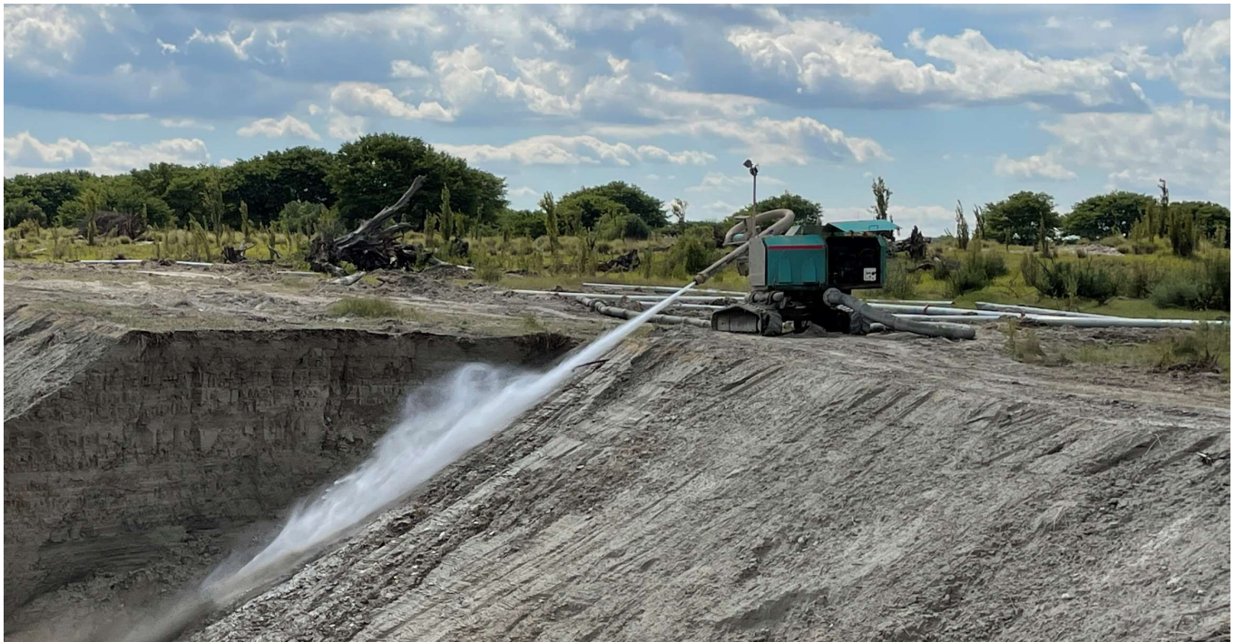
Figure 17: Semi-autonomous track mounted hydro-mining mining unit, top-down mining method (Source: Fraser Alexander)
