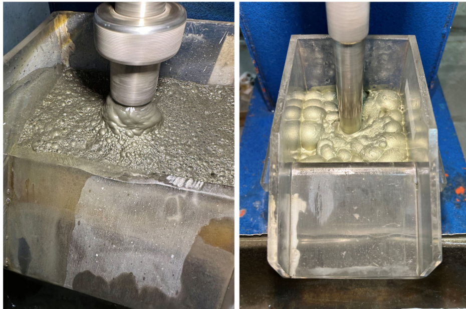
Figure 7. Photographs showing desktop rougher (left) and cleaner (right) froth flotation test work on a mineralised composite from the Corvette Prospect conducted by ALS Metallurgy in Burnie, Tasmania (ASX MAG 30 May 2023).
