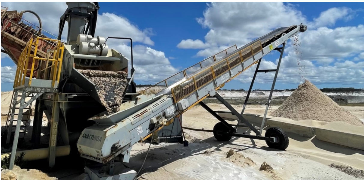
Figure 5: Third party Sand Wash Plant processing 20-tonne bulk sample from Stockyard Silica Sand Project
