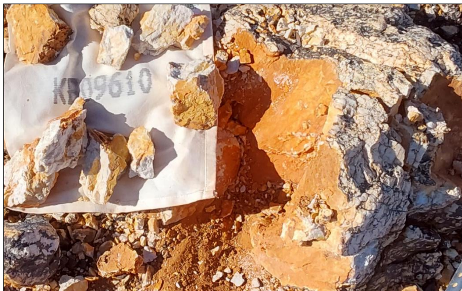
Photo 2 – Quartz vein outcrop rock chip resample returning 39.4g/t gold (KB09610), originally returning 22.5g/t gold rock chip assay (KB09374). Comprised of milky white, slightly bucky and brecciated vein quartz, with stockwork iron in fractures throughout and some limonite. Sample bag is 30 cm wide for scale.
