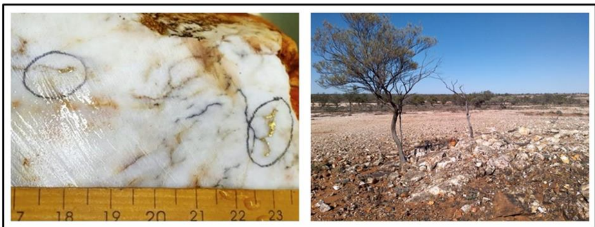
Photo 1. Visible Gold (circled) in historical sample of cut quartz vein (left) from outcrop (right) (4) . Scale of slab is in centimetres. Outcrop photo is looking west.
