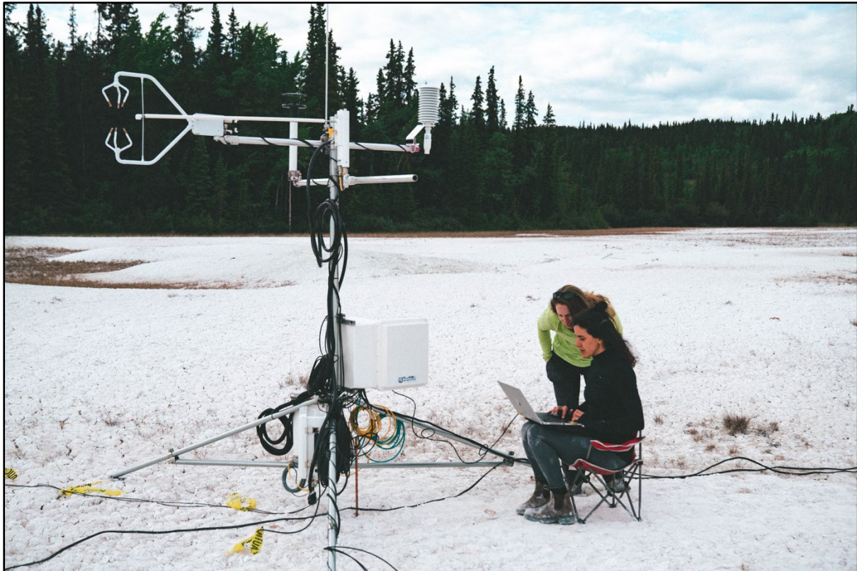
Figure 1: Arca scientists demonstrate how carbon dioxide mineralisation rates are measured on mine tailings. Photo: Taku River Tlingit First Nation traditional territory, British Columbia, Canada
