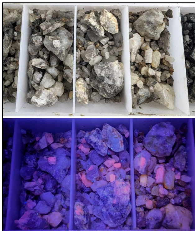
Figure 4: FSIR0010 chip trays from 43 – 46m downhole depth. Natural light (top) vs ultraviolet (UV) light at 365nm (bottom) showing spodumene crystals glowing pink under UV light.
