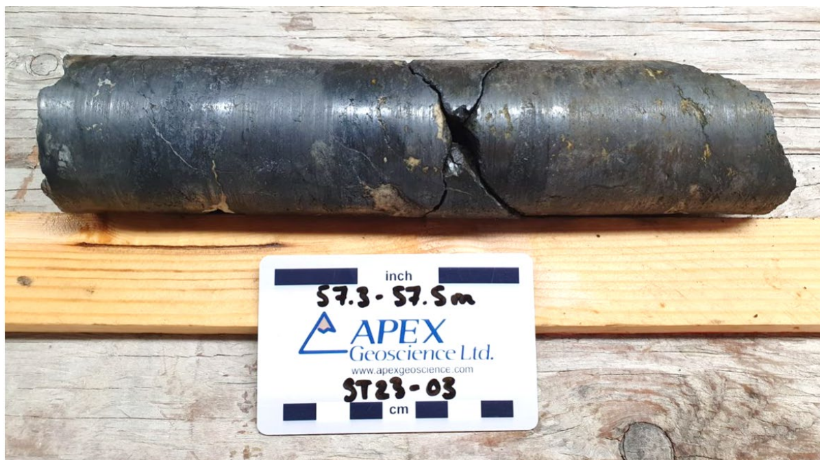
Figure 6: Massive chalcocite (dark grey)) in drill hole ST23-03 from approximately 57.4m downhole.
