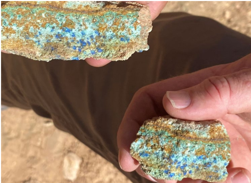
Figure 16: Rock samples showing heavily disseminated azurite (blue mineral – derived from oxidised chalcocite) from outcropping Dakota Formation within the Copper Warrior Project.
