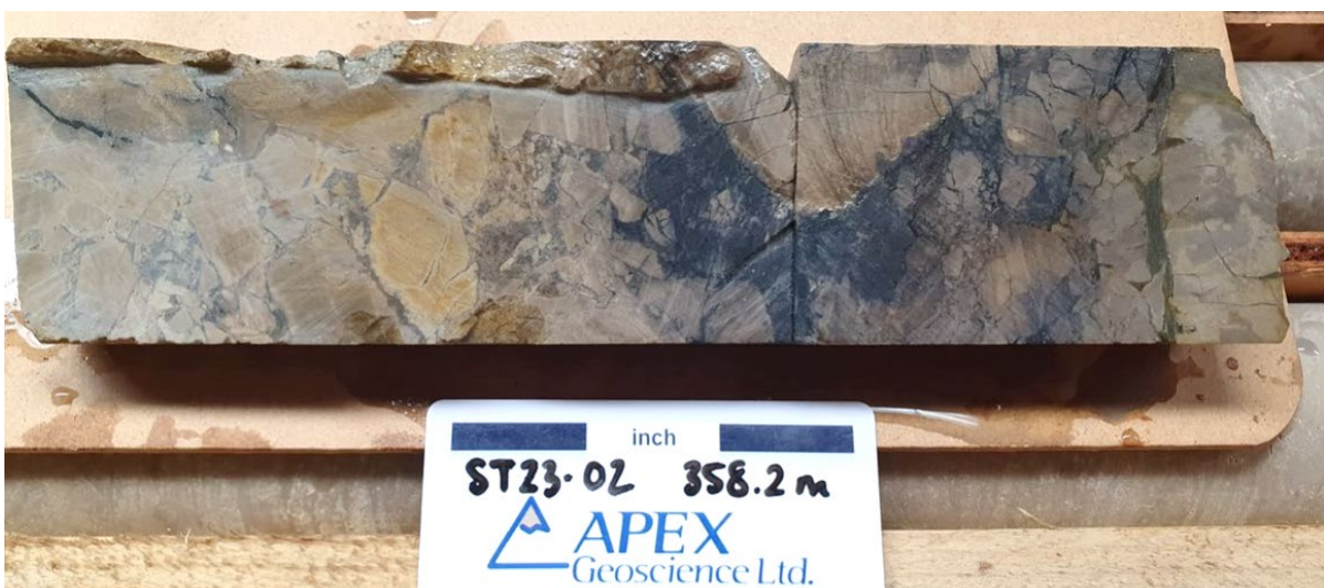
Figure 4: Strong chalcocite (dark grey) breccia fill and veining in drill hole ST23-02 from approximately 358.2m downhole. This interval assayed 2.7% Cu.
