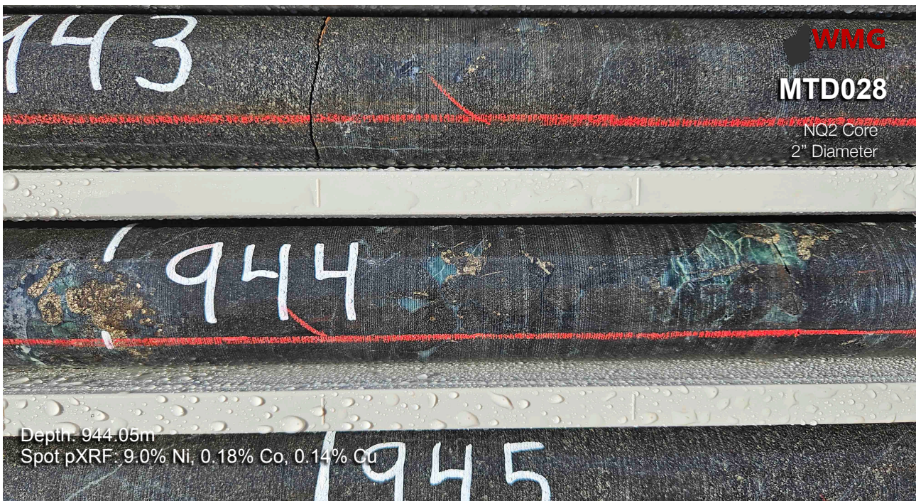
Figure 1: Photos showing examples of remobilised massive veinlets in hole MTD028 Note: core is NQ2 being 2 inches or 50mm diameter
