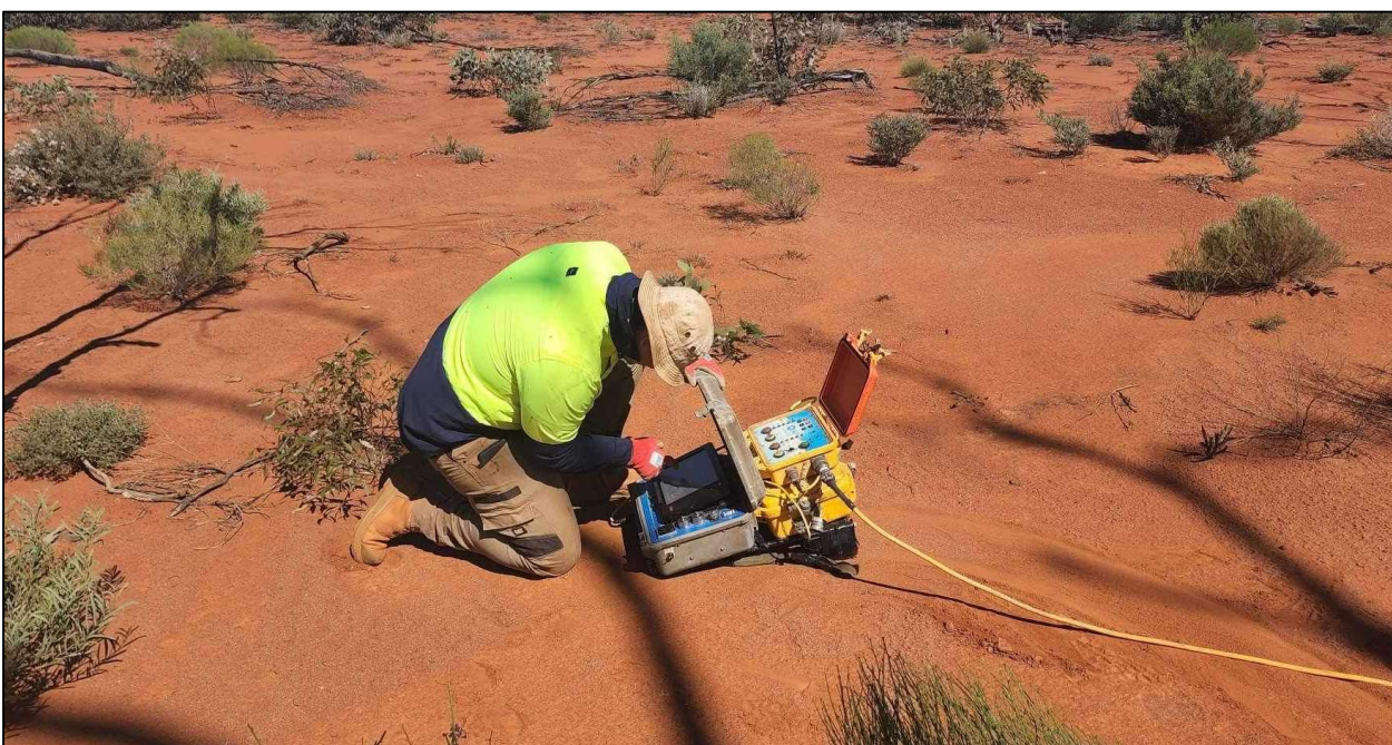
Photo 1: HPFLTEM survey underway at Octagonal
