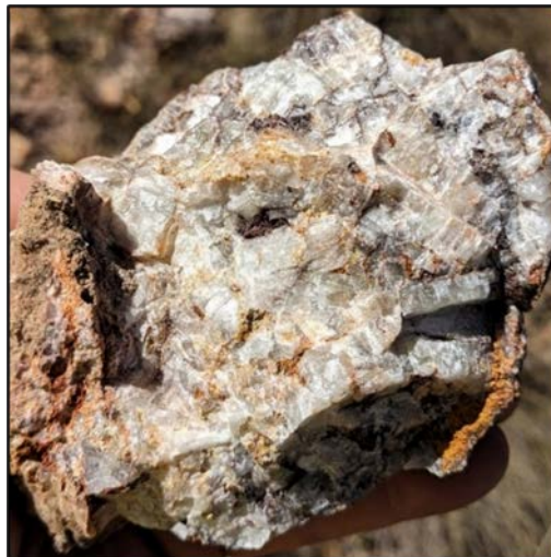
Figure 2: Barite, quartz and remnant sulphides in veining from Coronation Cu-Au (CO23_002, 1.91 g/t Au & 27 g/t Ag).
