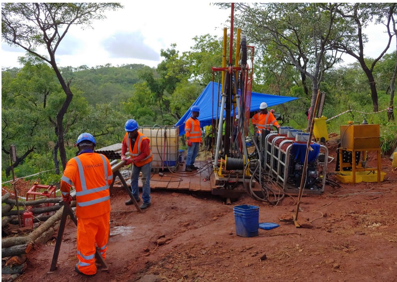
Photo 2. Diamond drilling to test the subsurface geology and geochemistry beneath a high-grade haematite outcrop at the Kowouleni target where a rock chip sample collected returned an assay in excess of 64% Fe.
