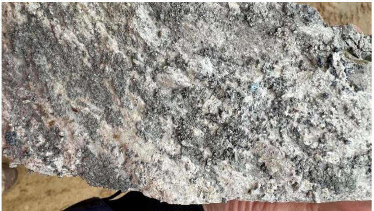
Pyrite + muscovite + nontronite on broken core surface. 89.25m.
