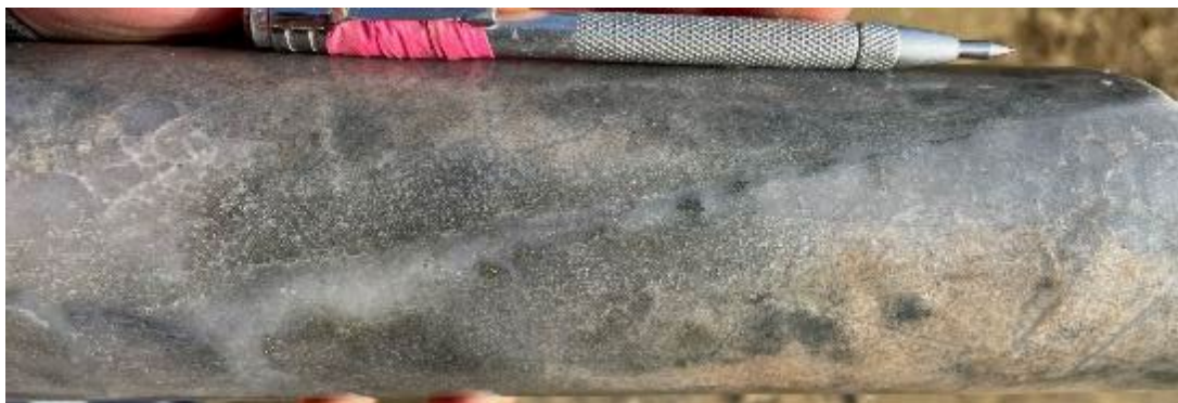
Intense sericite+silica+clay+pyrite alteration selvage to quartz+pyrite vein in sandstone at 584.3m
