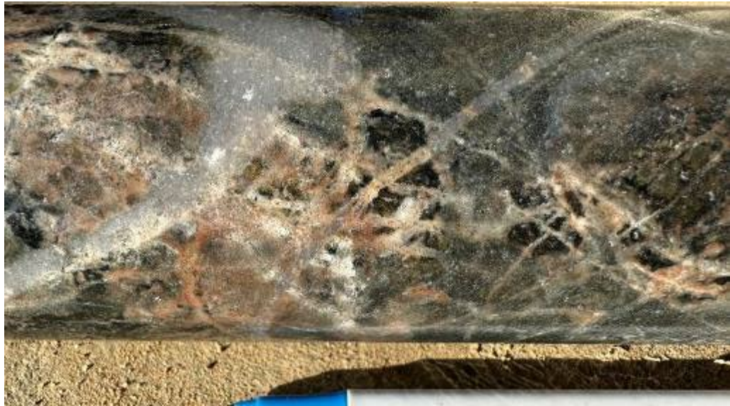
Vein Breccia with stockwork quartz veins with albite and chlorite-sericite patches. 393.8m.
