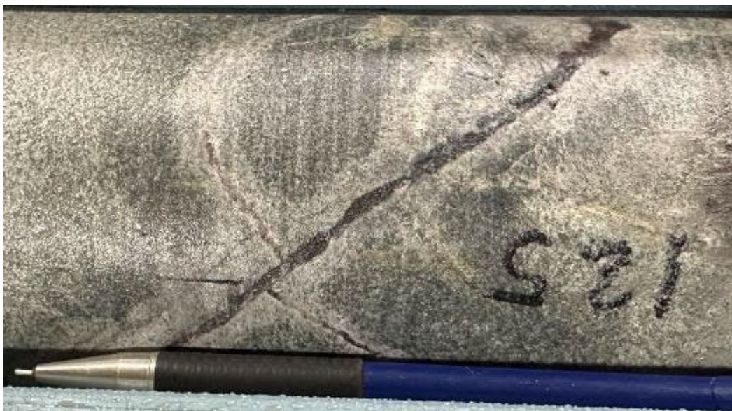
Magnetite vein in sandstone. 125m.
