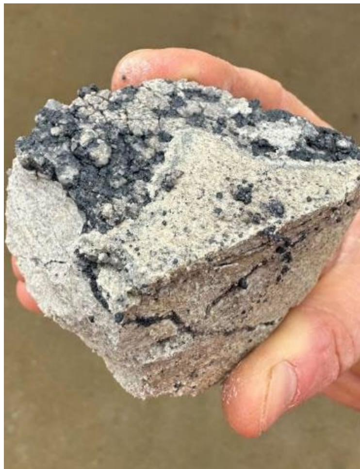
Chalcocite stockwork veins in clay-altered sandstone. 58.4m.
