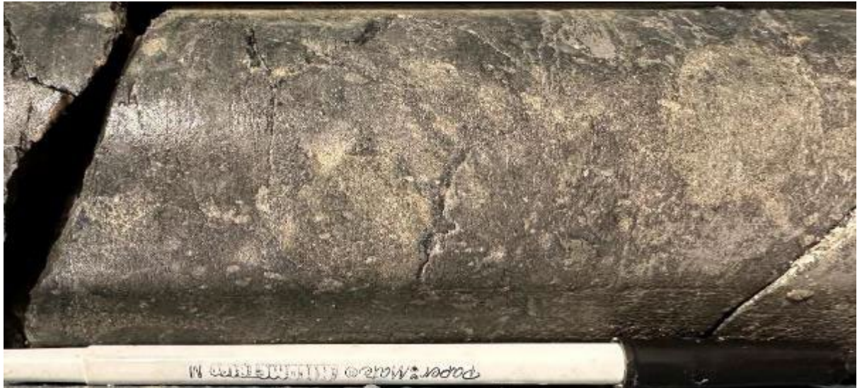
Breccia. Sandstone clasts in dark grey pyrite+clay-rich matrix. 99.3m.
