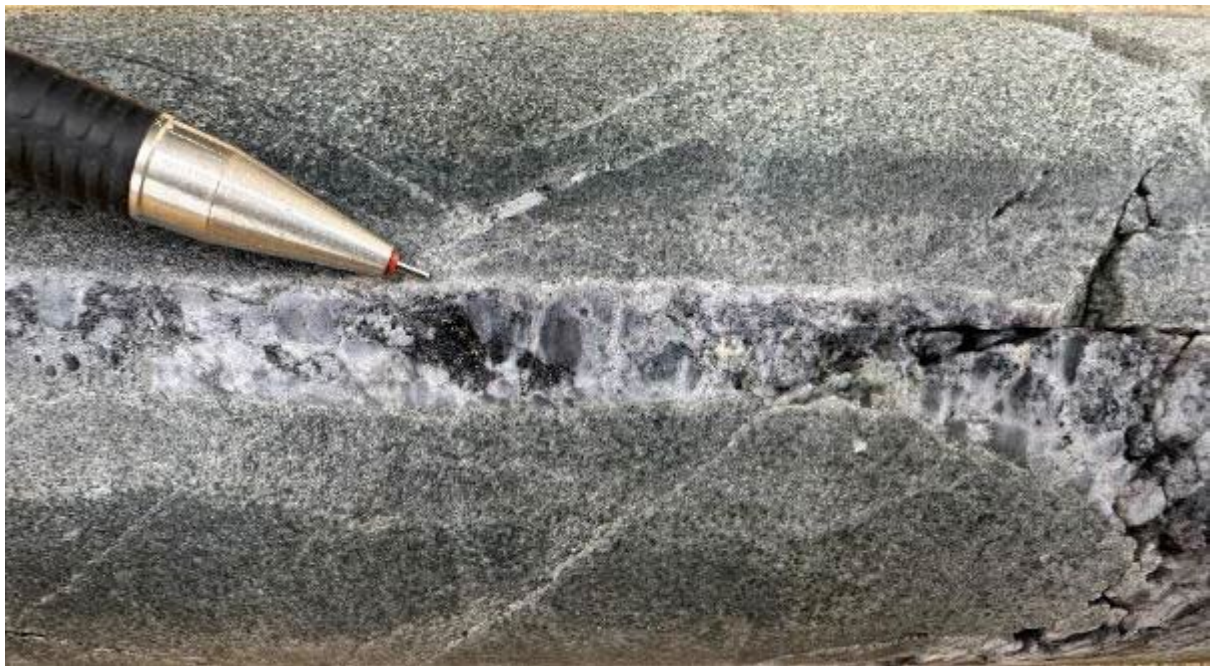
10mm wide quartz+magnetite+?biotite vein. Very coarse grained and sugary quartz and flaky magnetite. 139.35m.
