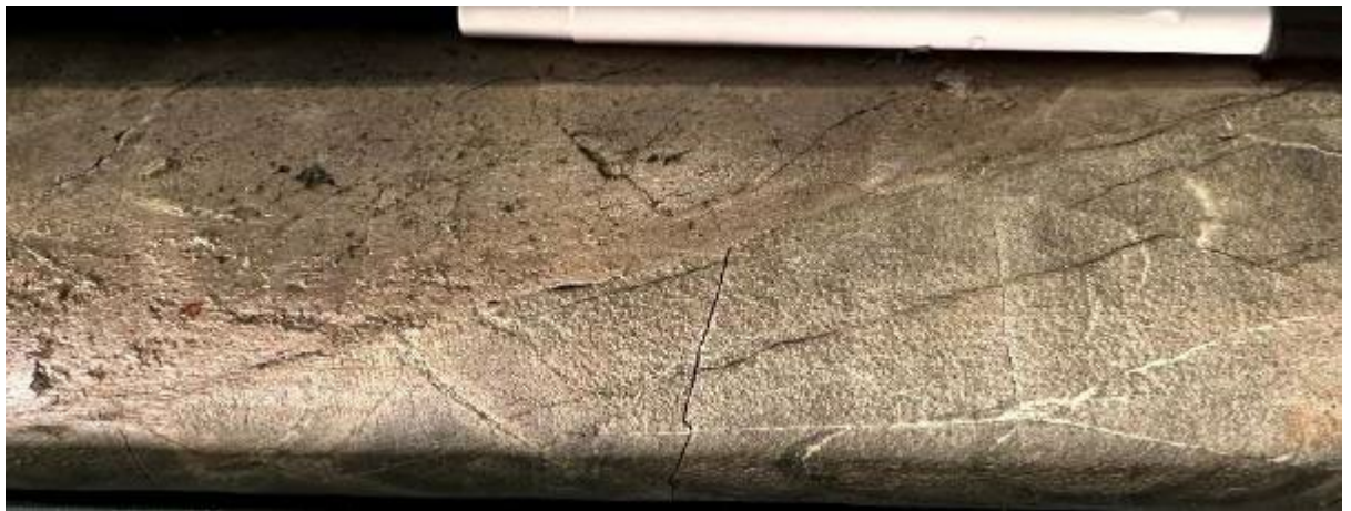
Downhole contact of microgabbro dyke with sandstone. 103.6m.
