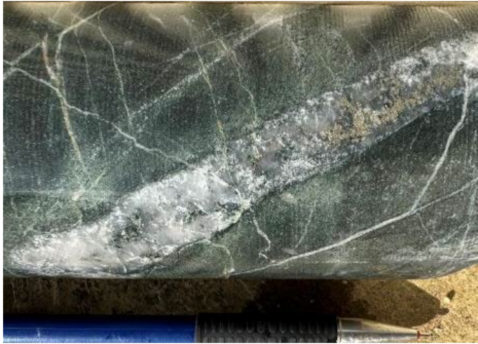
Quartz+carbonate+pyrite vein with rare chalcopyrite. 323.1m.
