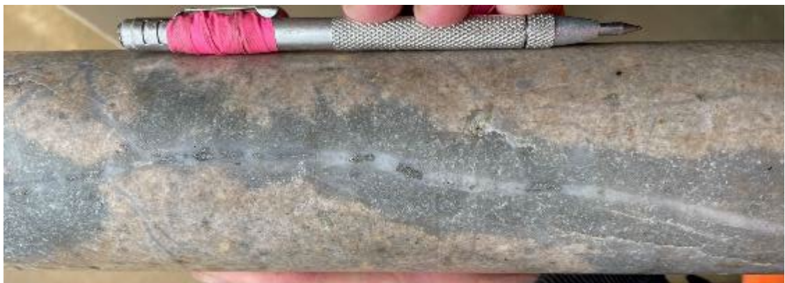
Quartz+pyrite vein close to core axis with strong sericite alteration selvage in microgranite at 565.3m
