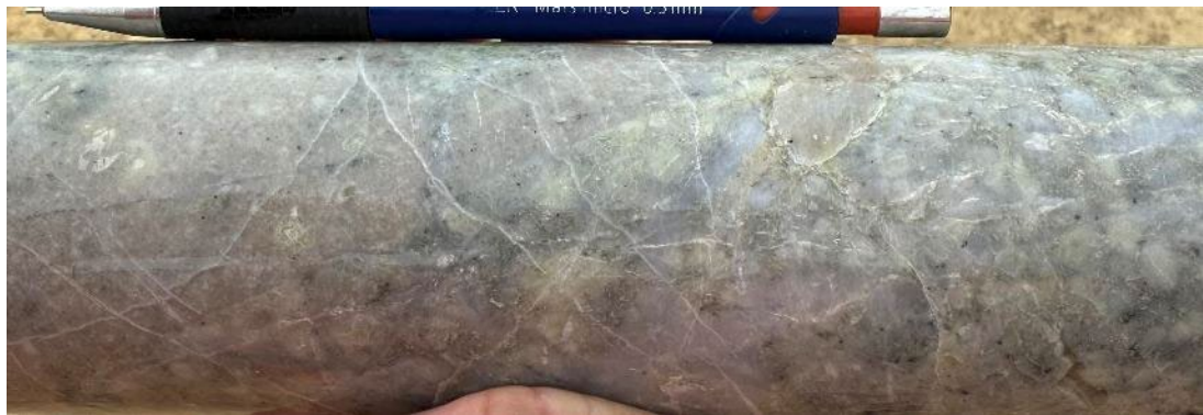
Contact between microgranite (left) and sericite-altered dacite porphyry (right) in the immediate hangingwall of the Low Angle Structure. 716.0m.
