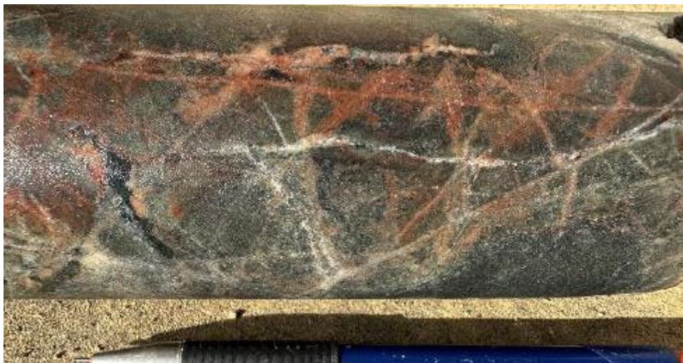
Quartz±carbonate veins and chlorite stringers with patchy hematite and/or sericite selvages. 374.6m.
