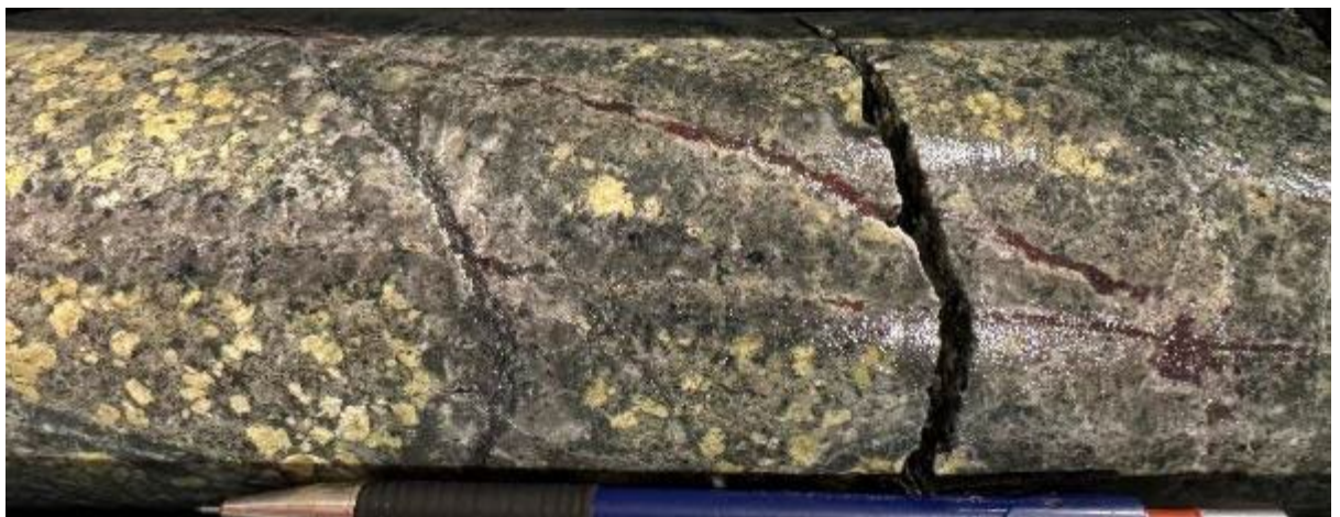
Dacite porphyry with moderate to strong pervasive sericite. Cut by chlorite and hematite veinlets with sericite selvedges. 176.7m.
