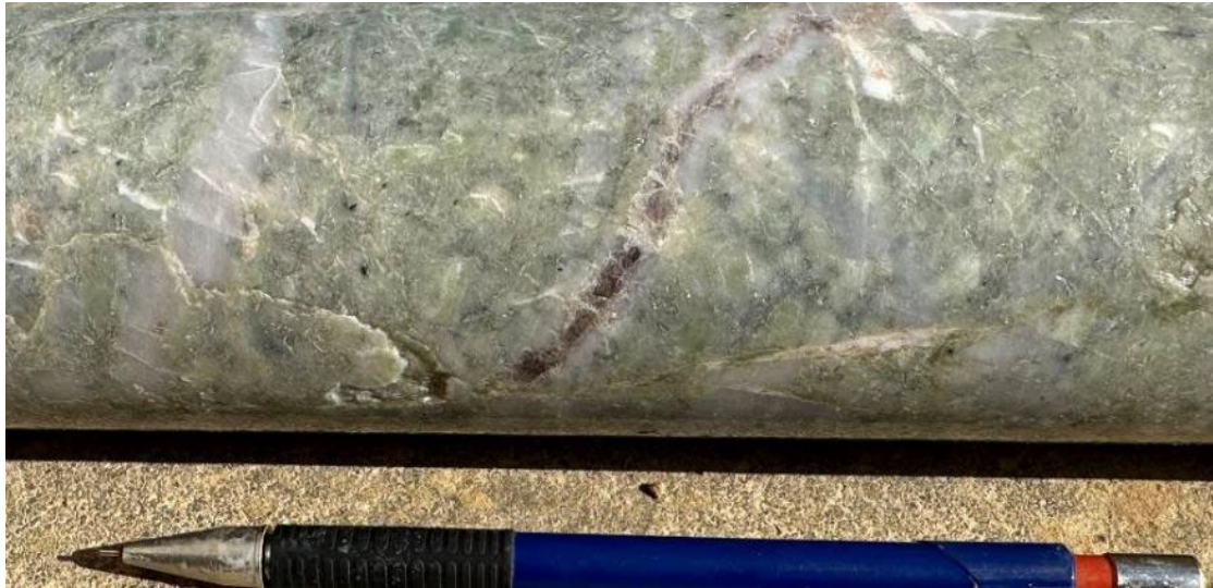
Quartz vein with anhydrite centre seam (centre of photo) in strong to intensely sericite-altered dacite porphyry. 714.6m.
