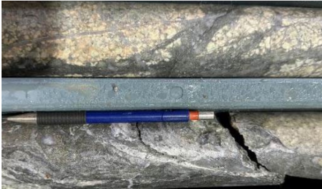
Quartz+sericite+clay+pyrite veins in very coarse grained dacite porphyry. 518.5-519.6m.
