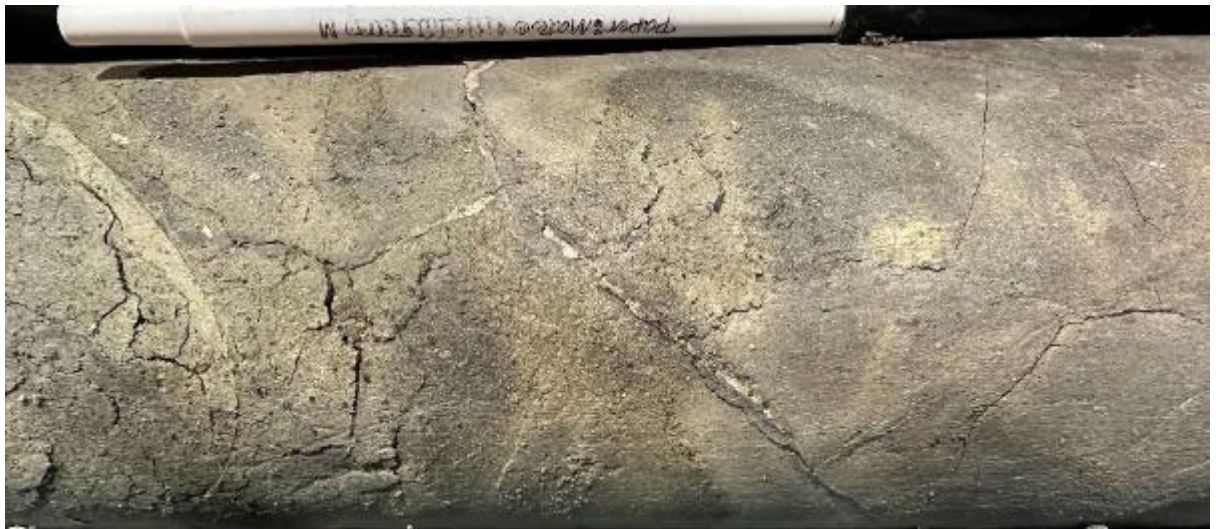
Microgabbro (left) and lamprophyre (right) dykes. Clear cross-cutting relationship showing the lamprophyre, on the right intruded the microgabbro. 98.3m.
