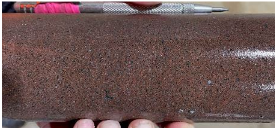
Hematite-carbonate-magnetite-hornblende rock at 287.7m.
