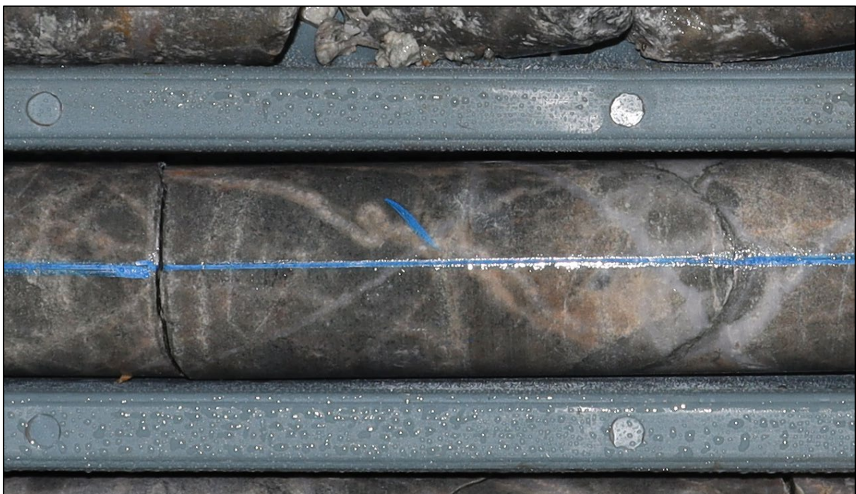
Photo 2. Drill core (HQ diameter) from 545m drill depth in SMD188 showing 'wormy' quartz aplite A-type porphyry vein.
