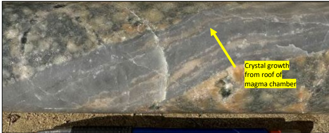
Photo 3. Wide laminated quartz vein with UST, 405.65m in SMD188.
