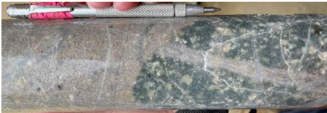
Microgranite/Dacite porphyry contact at 570.1m showing termination of earlier quartz vein hosted in Dacite Porphyry by microgranite intrusion.
