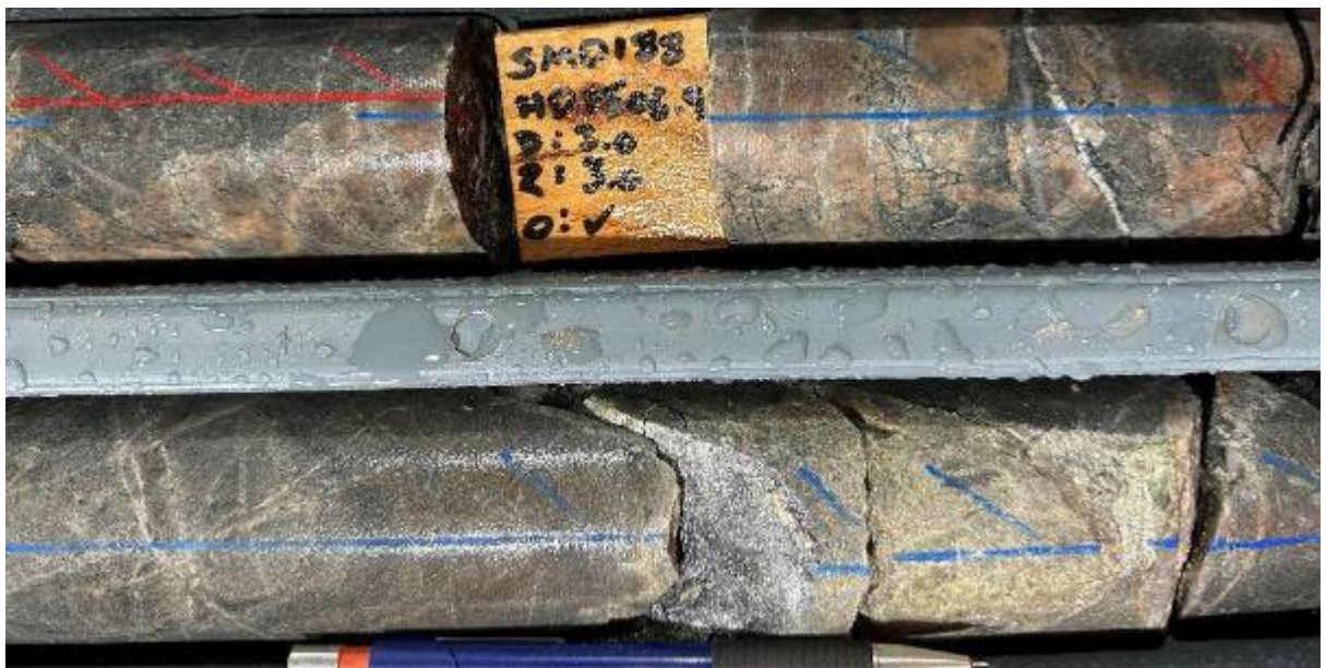
Molybdenite+pyrite on fracture with sericite selvage (bottom row). 507.7m.
