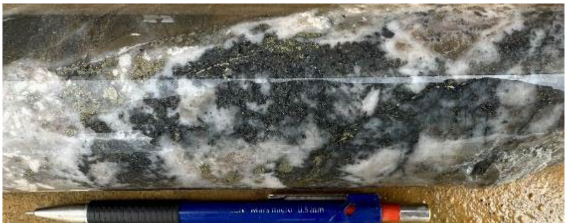
Large quartz+tennantite+chalcopryite+pyrite vein. 543.7m. pXRF showed Fe, Cu, Zn and As>>Sb.
