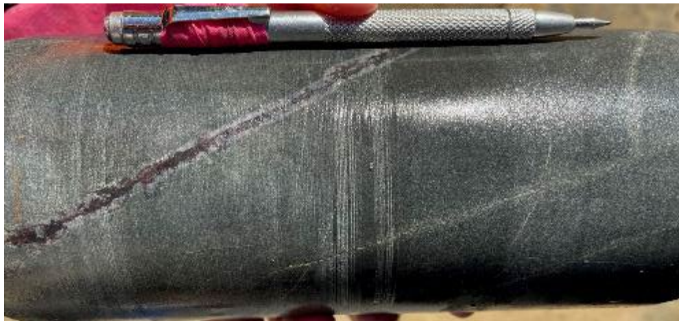
Quartz-magnetite-hematite vein (left) and fine quartz-chalcopyrite-chlorite veins in sandstone at 198.8m.
