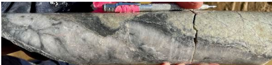
Sheared quartz+pyrite vein at 667.5m.
