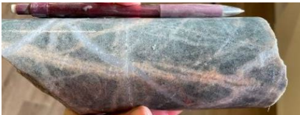
Early wavy quartz vein stockwork with albite-hematite selvages overprinted by later quartz veins in sandstone at 546.3m.
