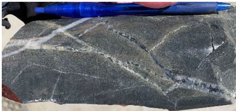
Quartz-magnetite-chlorite veins with trace albite and weak sericite-pyrite selvages and quartz vein in sandstone at 205.8m.
