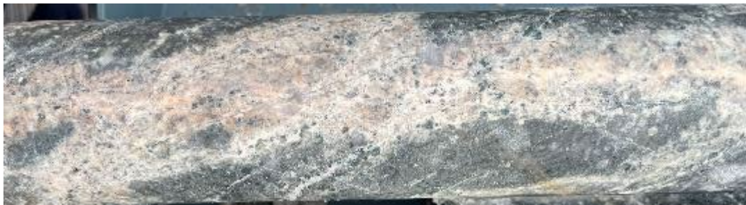
Quartz veinlets with sericite-(?)albite selvages in chlorite altered dacite porphyry at 249.3m.
