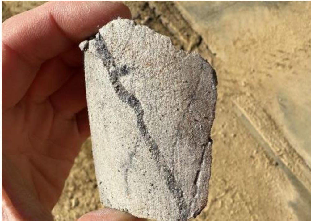
Pyrite D vein in clay-altered sandstone. 86.75m.
