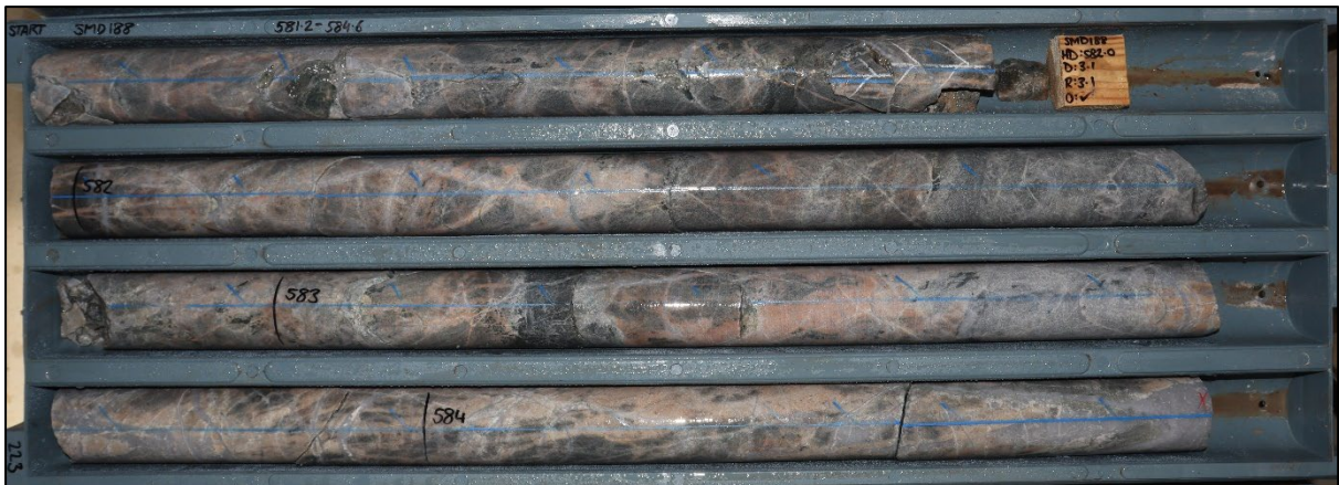
Photo 1. Drill core tray from 581.2m to 584.6m drill depth in SMD188 showing intense overprinting quartz and aplite veins/vein dykes.
