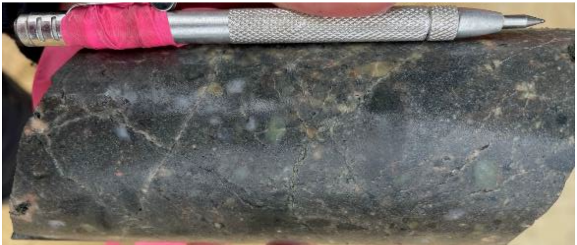
Dacite porphyry and minor sandstone (irregular contacts) at 265.5m.
