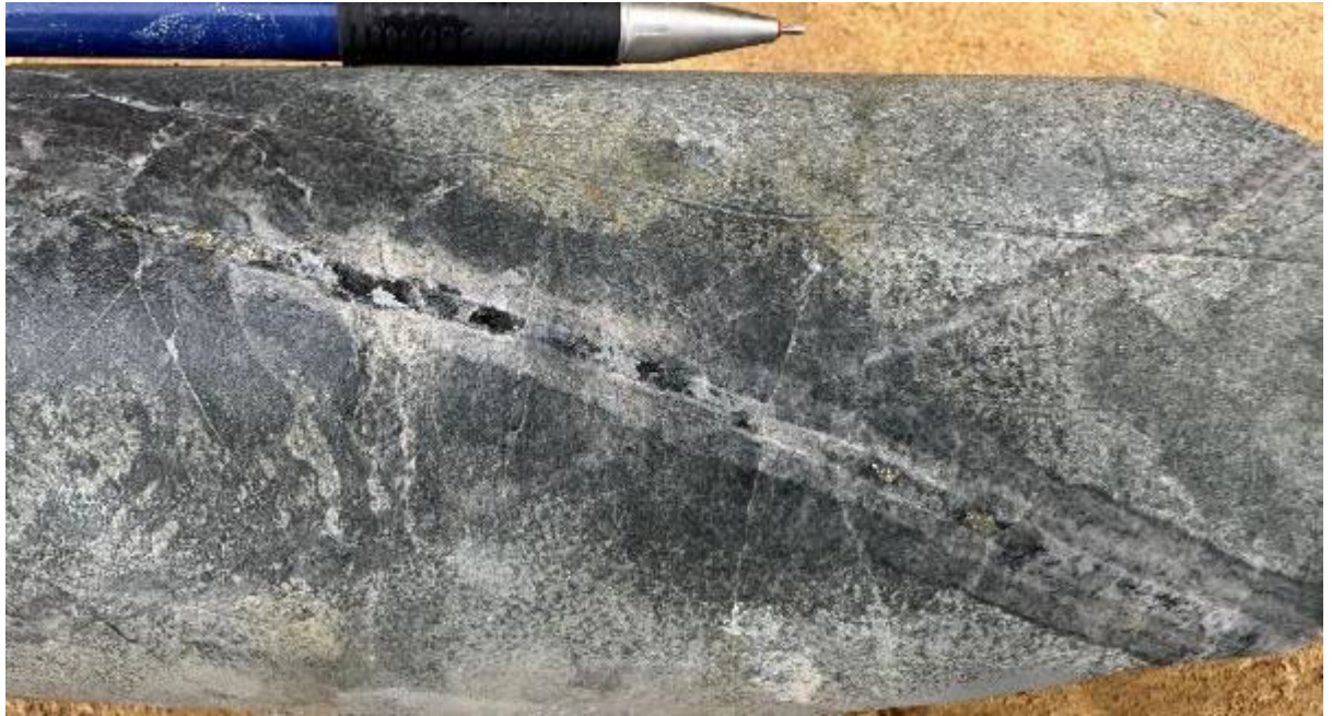
3mm wide quartz+magnetite+chalcopyrite+pyrite vein. Possible kfeldspar grading out to chlorite selvedge. 144.65m.
