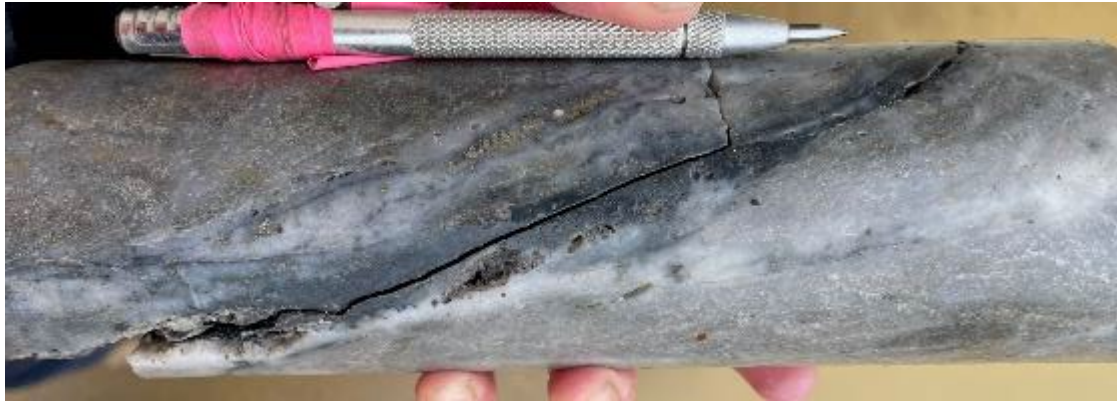
Quartz+pyrite+tennantite-tetrahedrite+chalcopyrite vein in sericite-silica altered sandstone at 559.7m.
