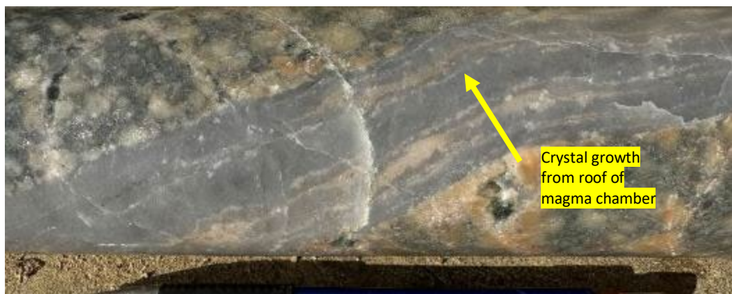
Wide laminated quartz vein with UST, oriented 72/005. 405.65m.
