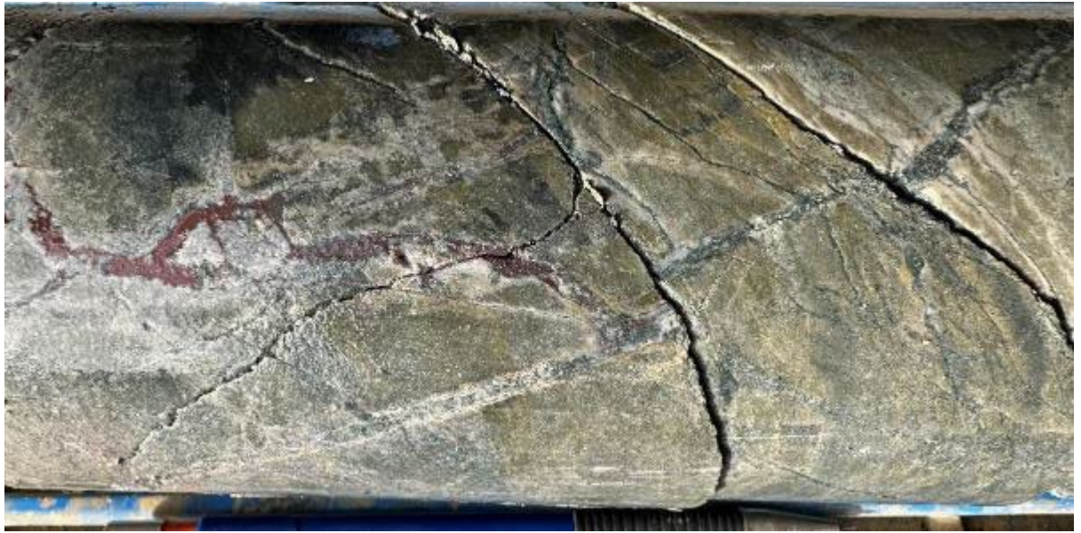
Sheared, sericite-altered sandstone cut by hematite and chlorite veins. 182.1m.
