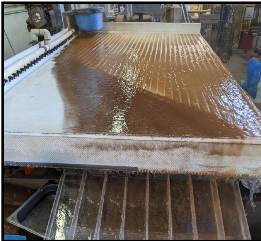
Figure 5: Laboratory Size Wilfley Table (View from Discharge End)
