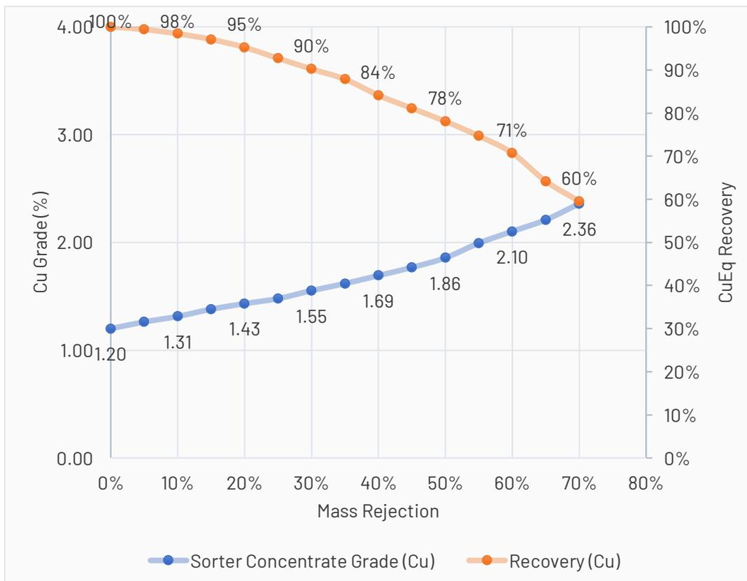
Figure 2 Ore sorter recovery and grade improvement on a copper equivalent (upper) and copper (lower) basis from simulated diluted ore at a simulated mined head grade of 1.87% CuEq, 1.20% Cu.
