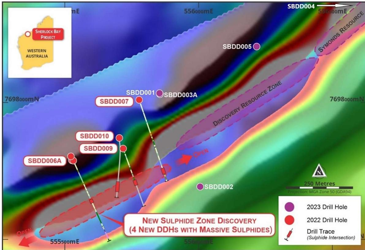
**Figure 2: New diamond drilling at Sherlock Bay which intersected a new sulphide zone with a strong EM conductors.**
