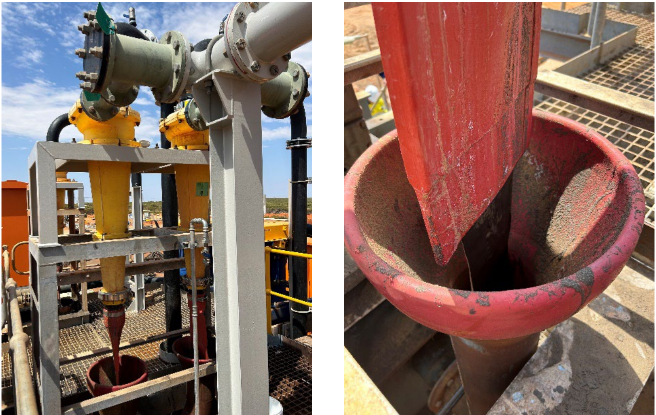
Figure 1. Modification to the mineral cleaning circuit included reconfigured feed cyclones to increase feed density
