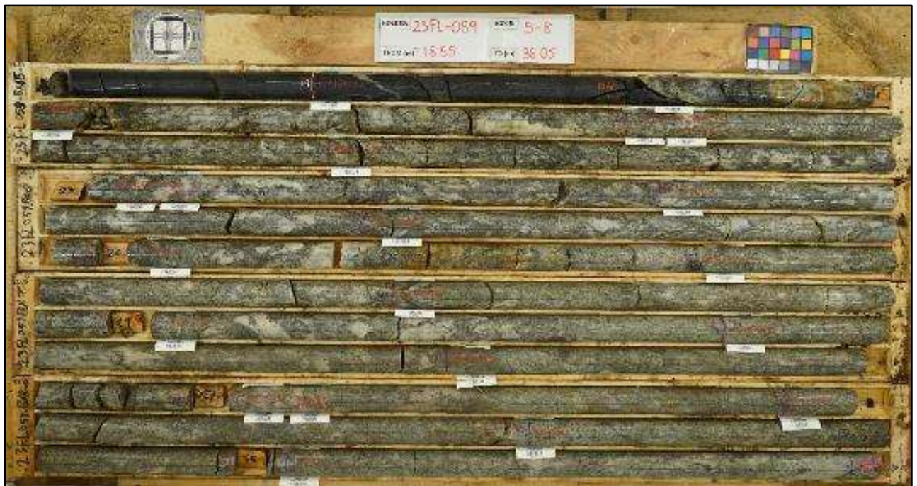
Figure 4 – Core box containing spodumene mineralisation in hole 23FL-059
