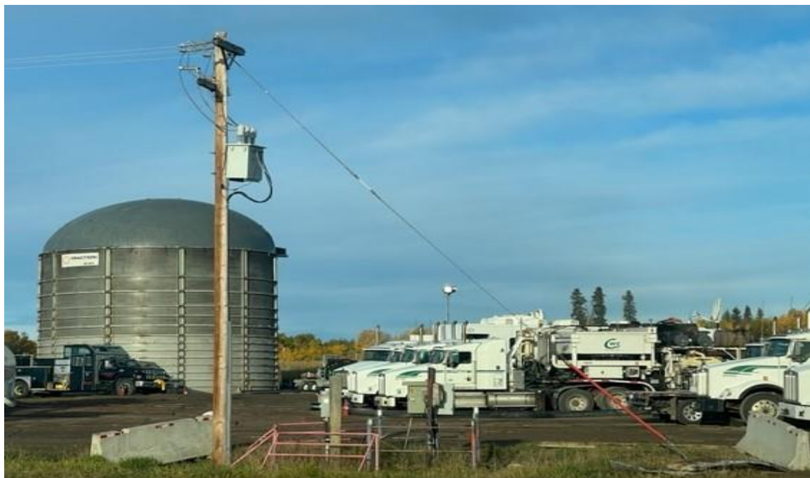
Figure 4. Completion Equipment on location – Pump Trucks and Water Storage for Fracture Stimulation.
