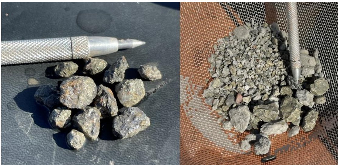
Figure 1 – EHRC733 sulphide examples and sieved Navajoh Unconformity Unit. Left: EHRC733 select sieved sulphide bearing samples from interval 159-160m showing coarse sphalerite, galena, and pyrite. Right: EHRC733 sieved Navajoh Unconformity Unit host lithology chips from 165-166m
