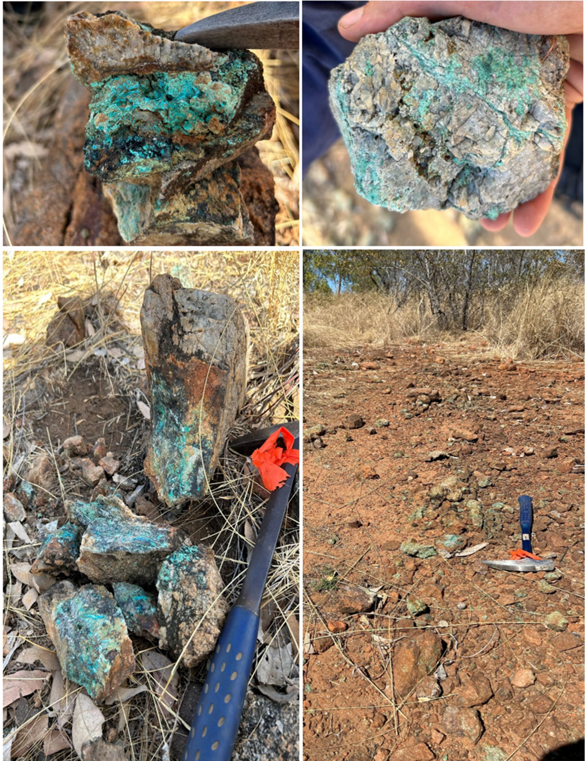
Figure 1. Samples from the extensive outcropping secondary-copper mineralised veins in the Fiery Creek tenement
