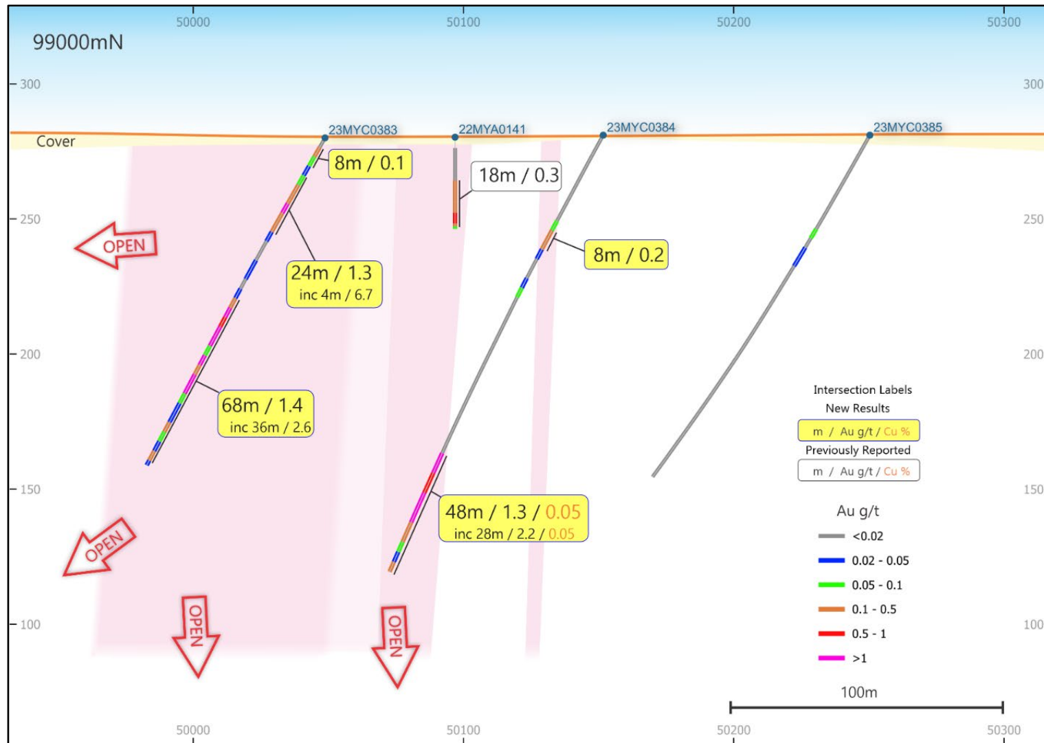
Figure 3: GEO-01 prospect stacked cross-section 99,000mN showing first-pass broad spaced RC gold-copper drill intercepts. NB: 50m elevation (RL) and 100m easting Local Grid co-ordinates, looking toward Local Grid 360° (or 328° MGA Zone 51 Grid).
