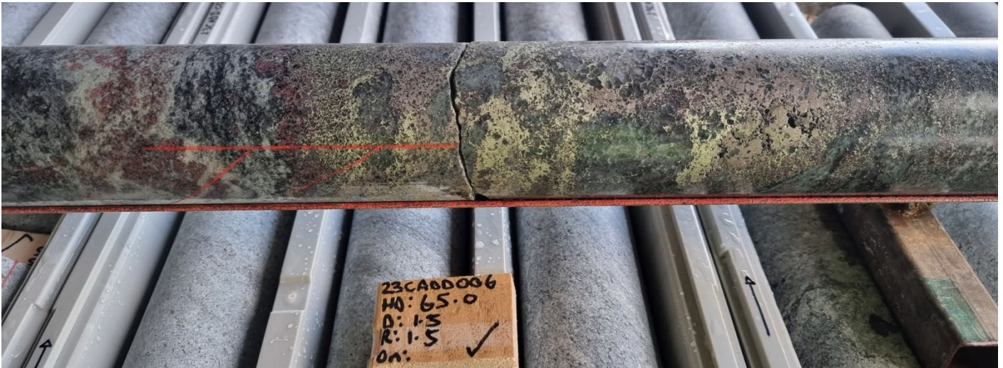
Figure 1: 23CADD006 65m, showing strong stringer chalcopyrite and pyrrhotite mineralisation associated with garnet
