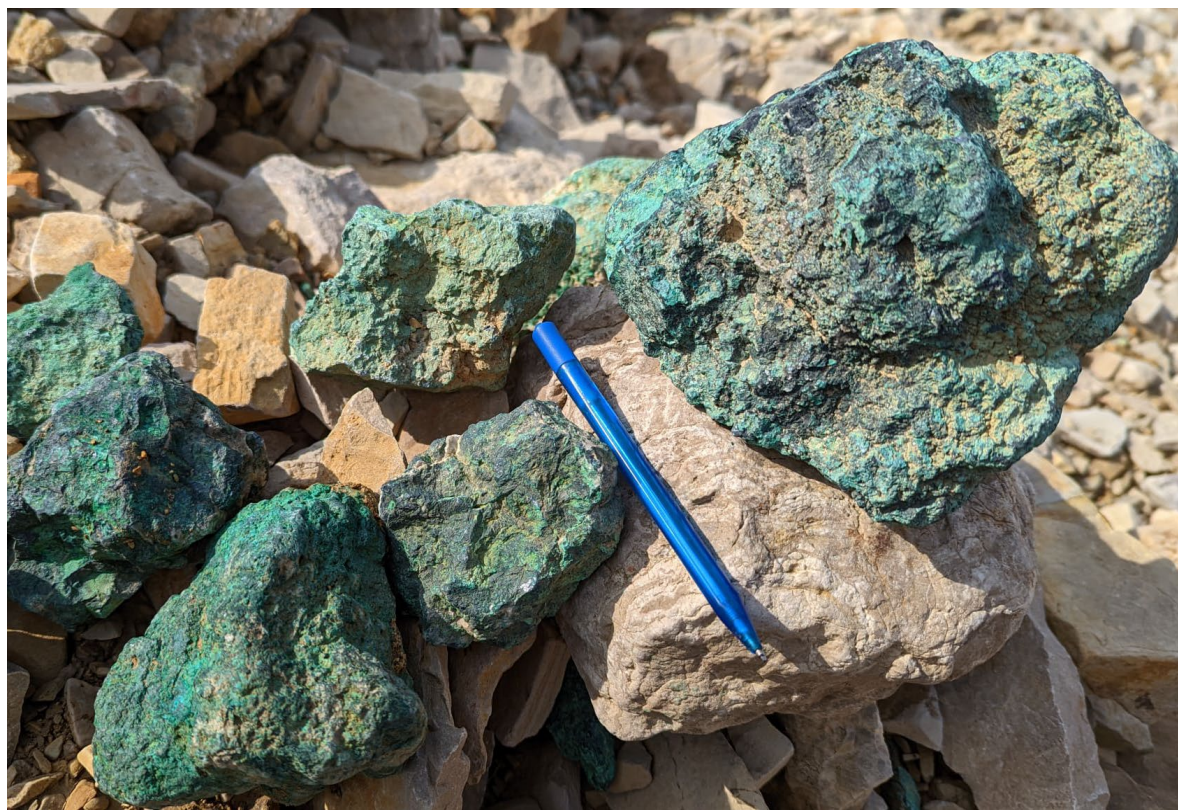
Figure 1: Massive chalcocite boulders exposed in the gully below the Lightning Ridge Prospect. The continued addition of new high-grade copper zones is significantly adding to the camp scale potential of the near-surface mineralisation at Storm. The average grade of chalcocite (copper sulphide) is approx. 79.8% Cu.
