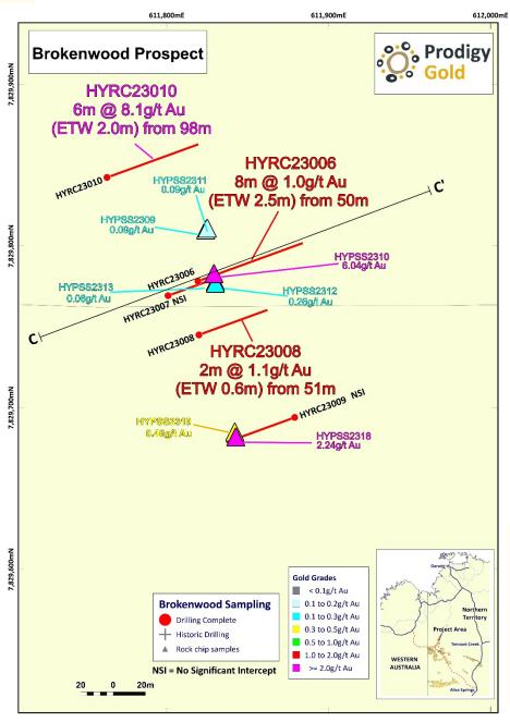
Figure 6 Plan showing sampling results<sup>5</sup> and drilling results for Brokenwood Prospect
