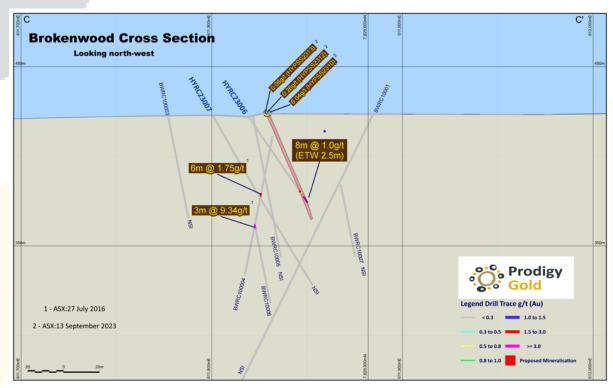
Figure 7 Cross-section of Brokenwood Prospect mineralisation showing results for holes HYRC23006 and 23007
