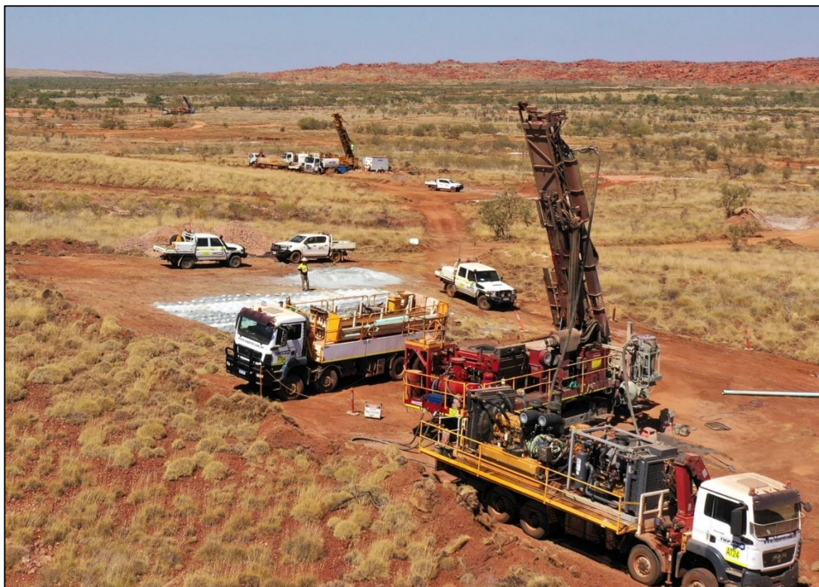
Figure 2 – Three rigs are now drilling at Tabba Tabba, two RC drill rigs and one diamond drill rig
