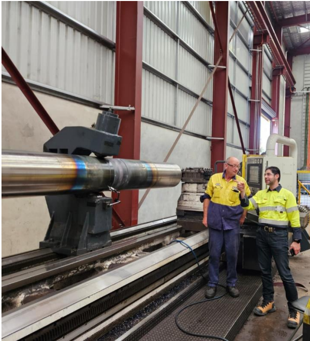
Hazer personnel inspecting final machining of reactor shell
