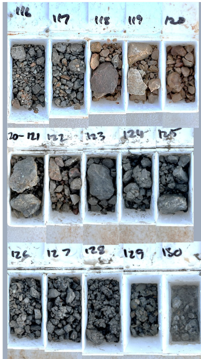
Image 1 –23STRC034 chip tray containing the interval between 115m to 130m.
