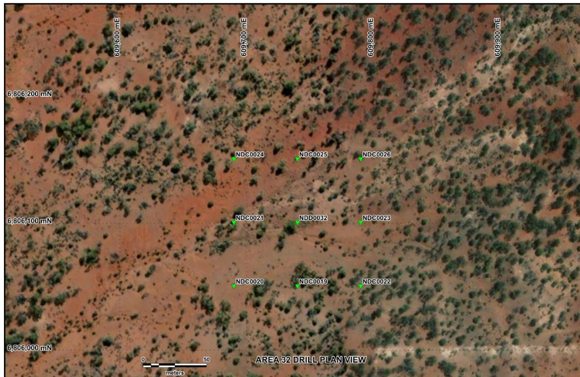
Figure 9: Area 32 drill locations with the RC holes around the diamond hole (NDD0032)
