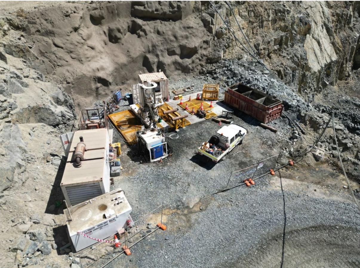
Figure 4 - View of the raisebore machine setting up to commence back-reaming the primary return air raise
