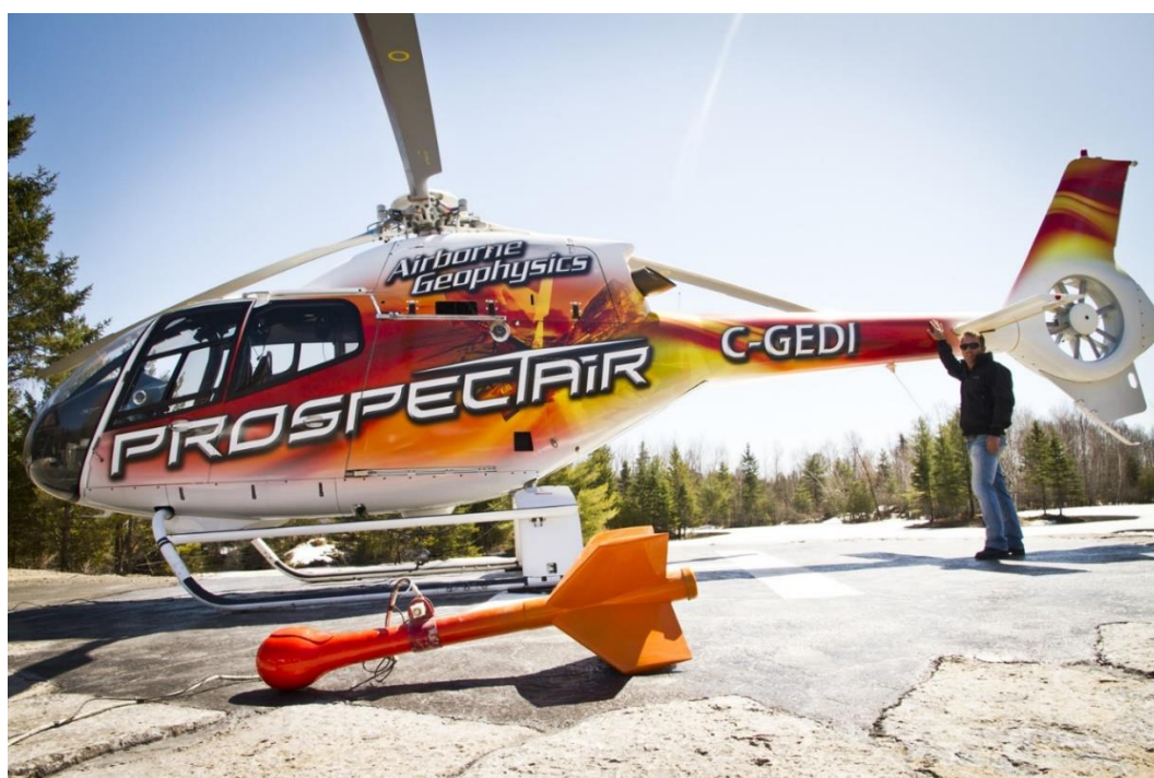
Figure 2 – Prospectorair magnetic and spectrometric survey helicopter and associated equipment.
