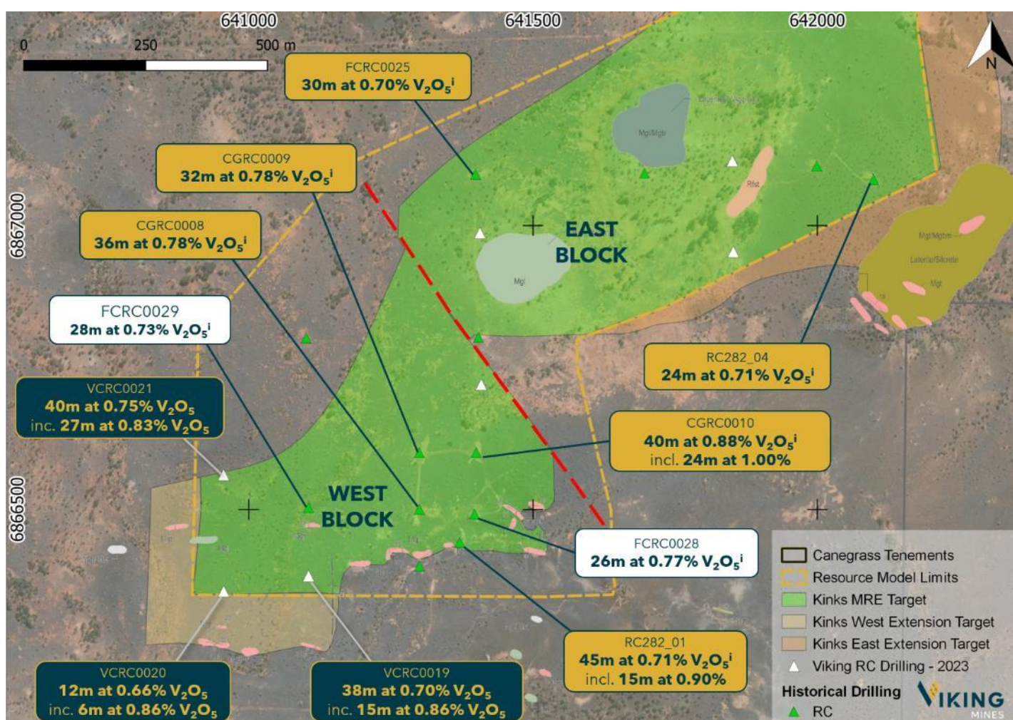
Figure 2 – Map of the Kinks Deposit and the Kinks West Extension ETE target area showing V_2O_5 assay results from Vikings 2023 drilling programmes. Intercepts are reported above a 0.5% V_2O_5 cut-off, with included intercepts (where reported) >0.8% V_2O_5 cut-off. Note historical drillhole results which have not yet been incorporated into the MRE for the Kinks deposit (orange callouts) and results currently informing the MRE (white callouts). 2
