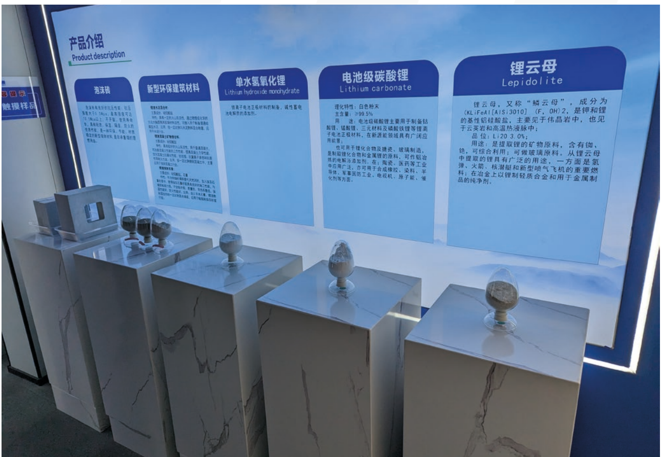
Yongxing display (right to left) of lepidolite concentrate and lithium products derived from lepidolite processing
