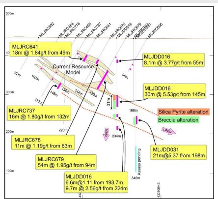
Lady Julie North 4 composite cross section showing open thickened high-grade dipping gold zone containing breccia and silica-pyrite alteration, upper mineralised zone and older resource model.
