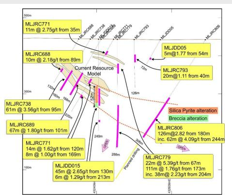
Lady Julie North 4 composite cross section showing open thickened high-grade dipping gold zone containing breccia and silica-pyrite alteration, upper mineralised zone and older resource model.
