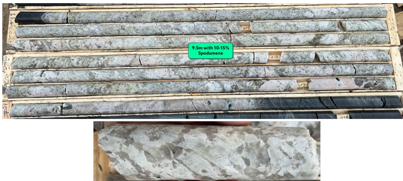
Figure 2: Abundant spodumene (10-15%) in drillhole AC-23-013. Inset: spodumene mineralisation up to 40% from 207.4m to 207.5m.
