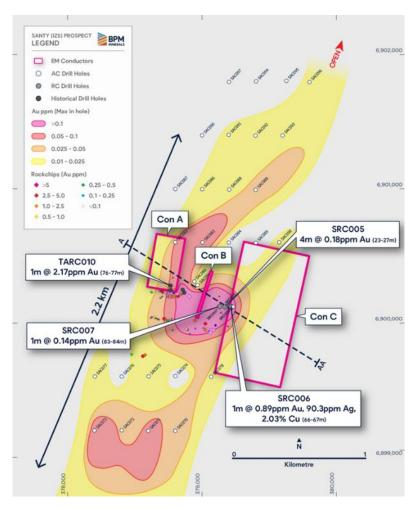
Figure 2 - Santy Project - IZ5 Prospect - FLEM Conductors
