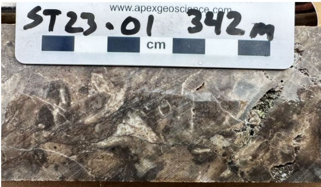
Figure 8: Chalcopyrite (brassy) in vugs and veinlets in drill hole ST23-01 from approximately 342m downhole.
