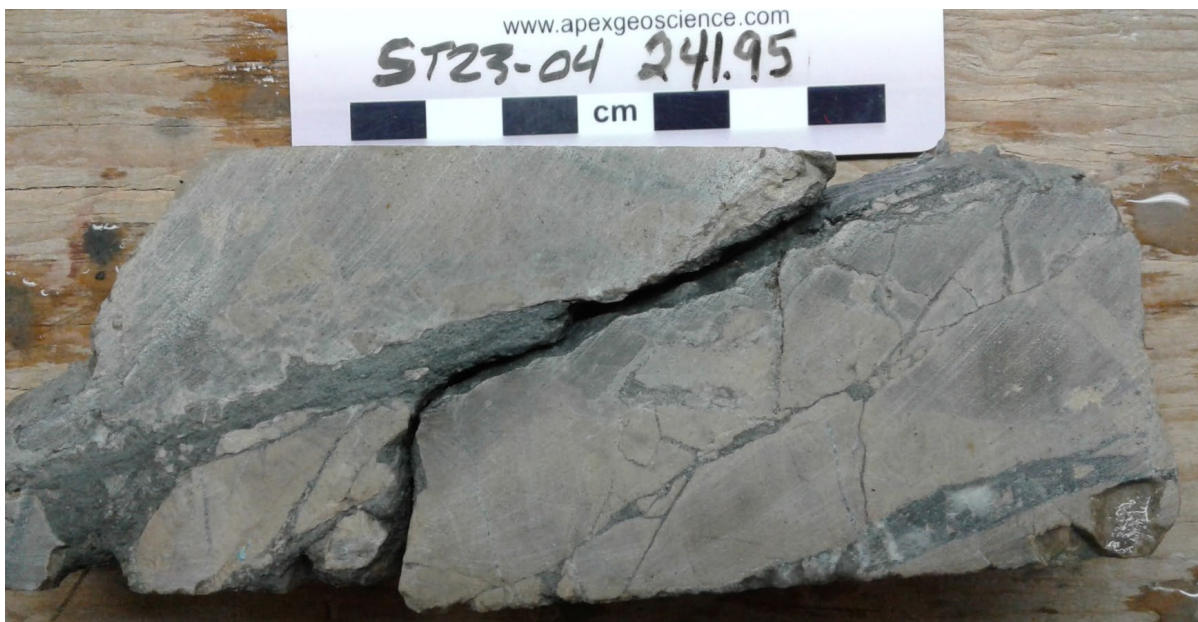
Figure 12: Silt and calcite (darker grey and white respectively) fracture fill within the Southern Graben Fault Zone from drill hole ST23-04 (approximately 241.95m downhole).
