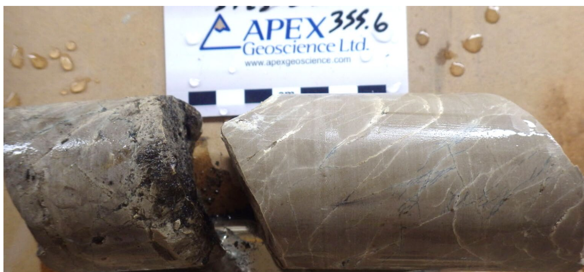
Figure 13: Breccia and veinlets of chalcocite (dark grey) in drill hole ST23-04 from approximately 355.6m downhole.
