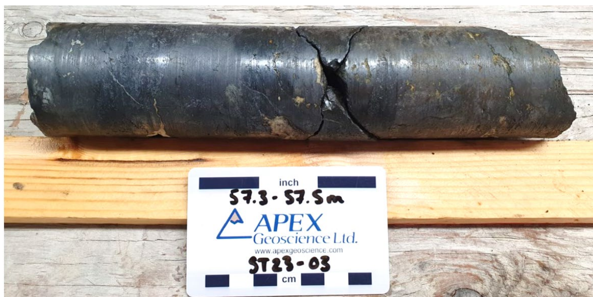
Figure 15: Massive chalcocite (dark grey) in drill hole ST23-03 from approximately 57.4m downhole. This is part of an interval of 57.2 – 57.7m @ 49.6% Cu.
