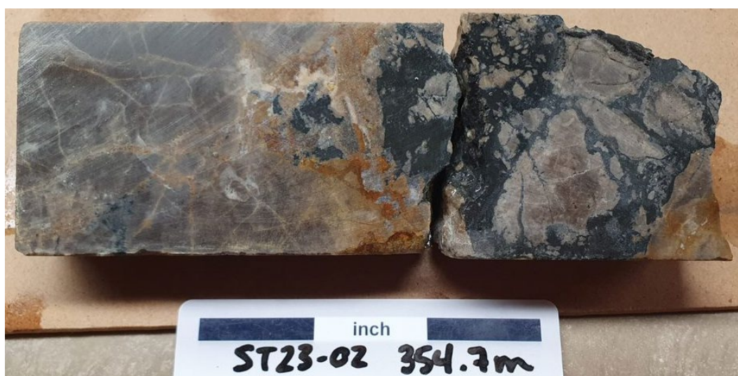
Figure 10: Chalcocite (dark grey) breccia fill in drill hole ST23-02 from approximately 354.7m downhole.
