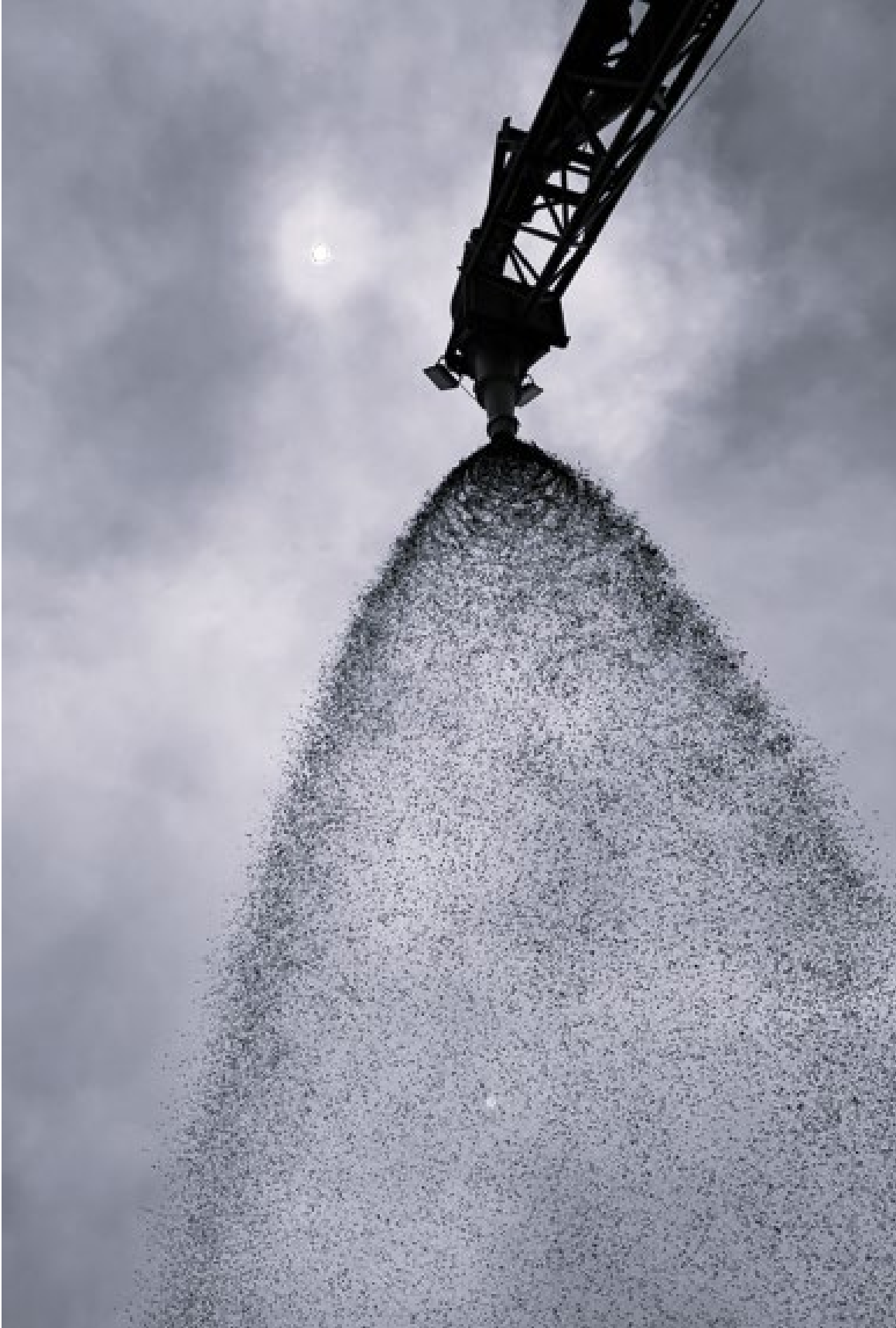
Image 6: Concentrate production at Thunderbird – cyclone discharge to stockpile
