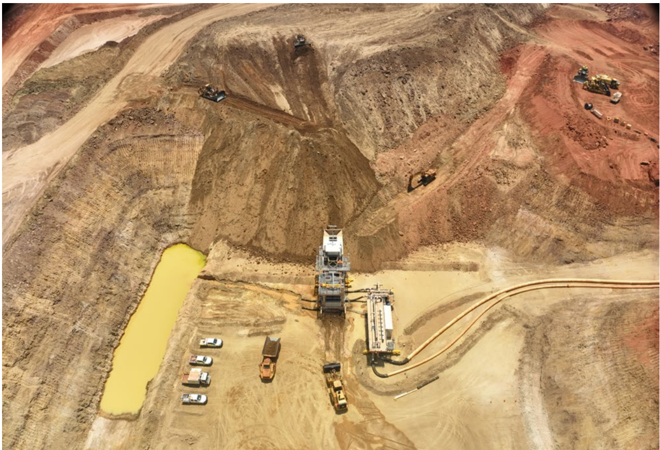
Image 3 & 4: Mining area with ore stockpile and DMU (above) & dozer push operations (below)
