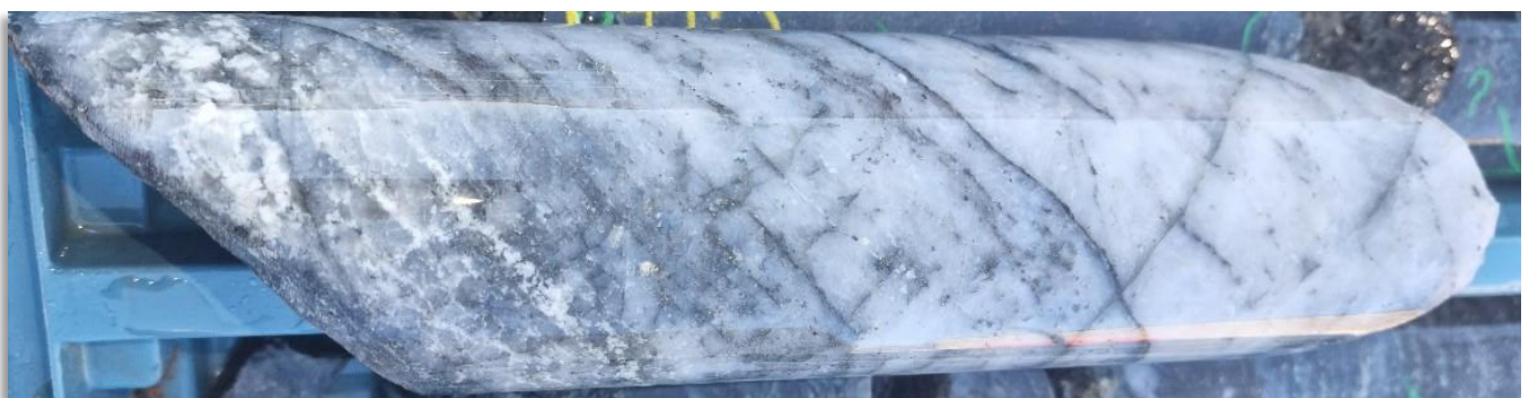
Figure 5: Drill core from SG23DD003 from 43.4m to 43.6m showing Norseman style quartz lode mineralisation with strong disseminated sulphide.
