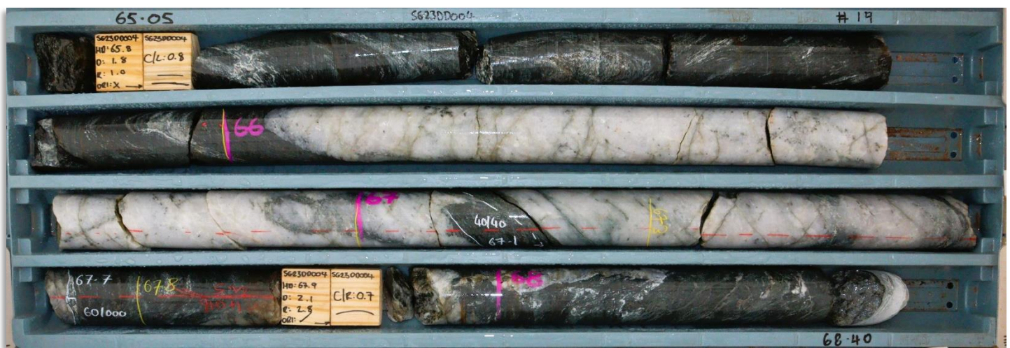
Figure 4: Drill core from SG23DD004 from 65.8m to 68.4m showing Norseman style quartz lode mineralisation with strong disseminated sulphide.
