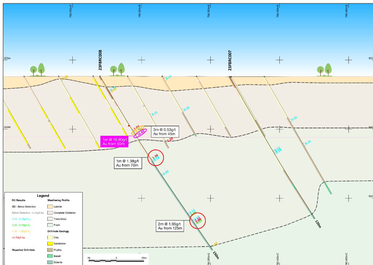
Figure 12: Cross-section of multiple mineralised intercepts recorded from 23FCRC008, which the company interprets has tested the fringe of a potentially large mineralised gold system.
