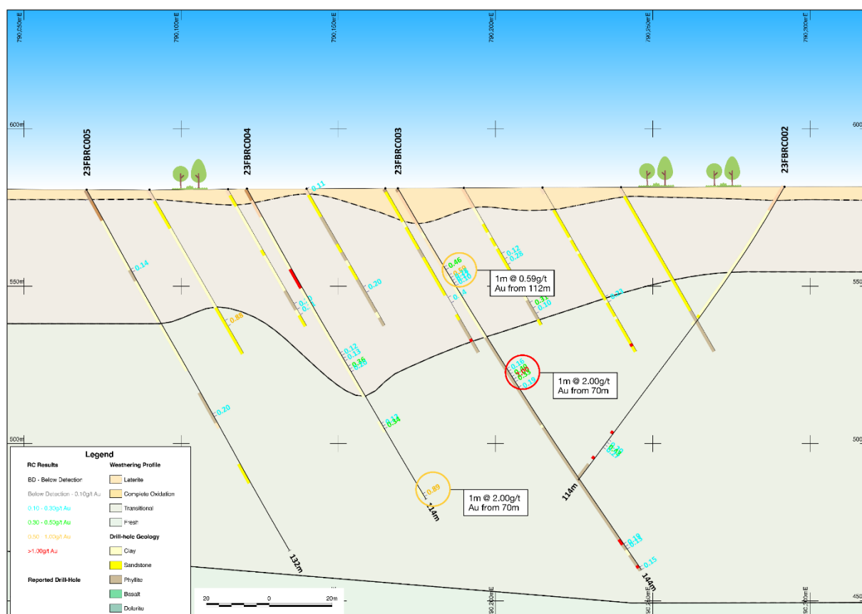
Figure 13: Cross-section of significant intercepts recorded in drill-holes 23FBR003 and 004.
