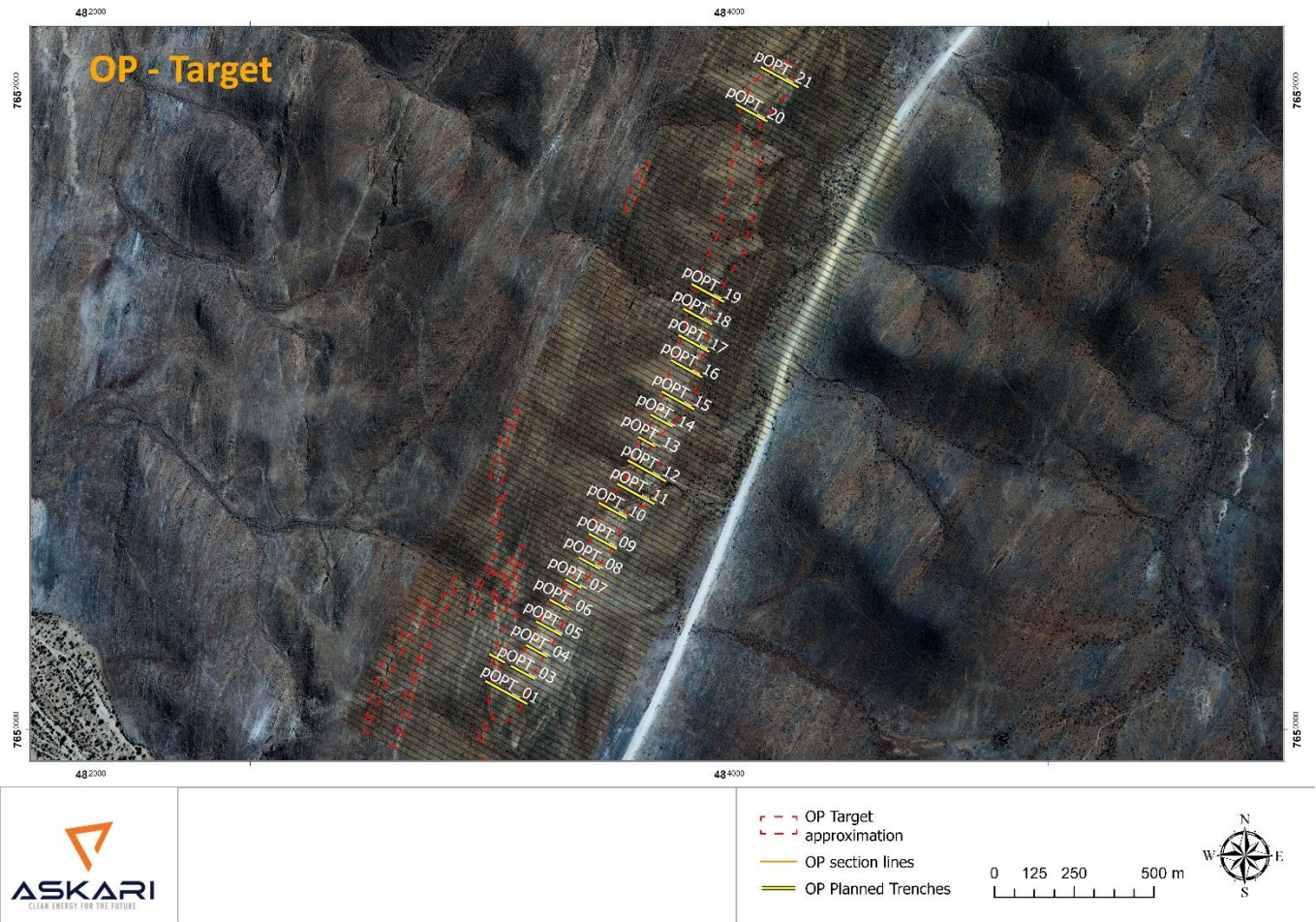
Figure 2: Planned Phase One trenches for the OP pegmatite.
