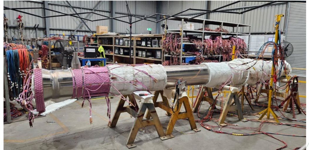
Reactor successfully heat-treated and preparing for final machining and assembly
