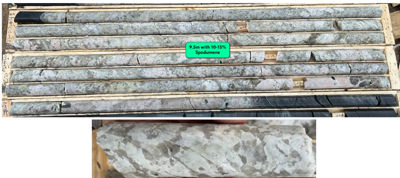
Figure 4: Abundant spodumene (10-15%) in drillhole AC-23-013. Inset: spodumene mineralisation up to 40% from 207.4m to 207.5m.
