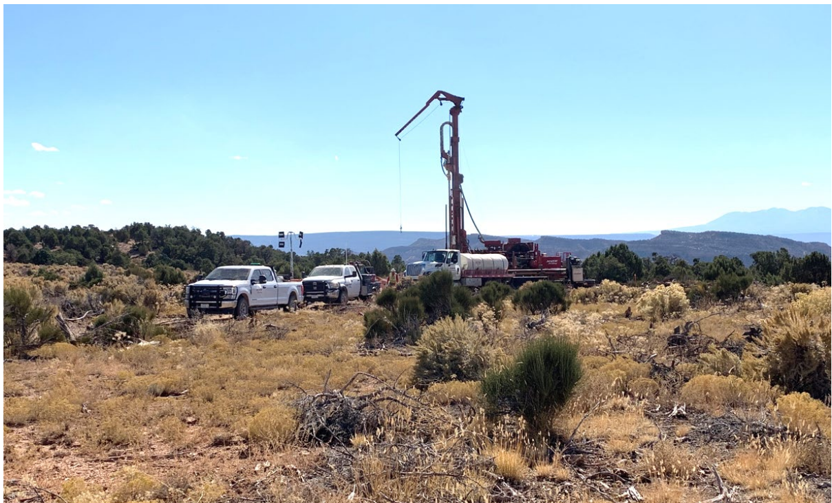
Figure 1: Reverse Circulation (RC) drilling rig underway at the Copper Warrior Project, Utah.
