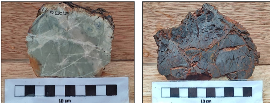
Figure 2: Rock slab from Au anomaly area in Sua Dum (left) calc-silicate rock crosscut by quartz vein/veinlet (right) Iron skarn with hematite ± quartz stained in fracture and trace of chalcopyrite
