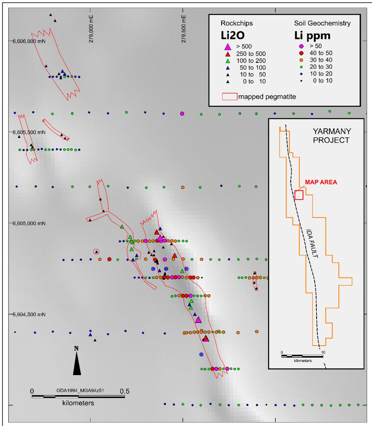
**Figure 1.** Yarmany Project F-camp prospect surface geochemistry over magnetics TMI
