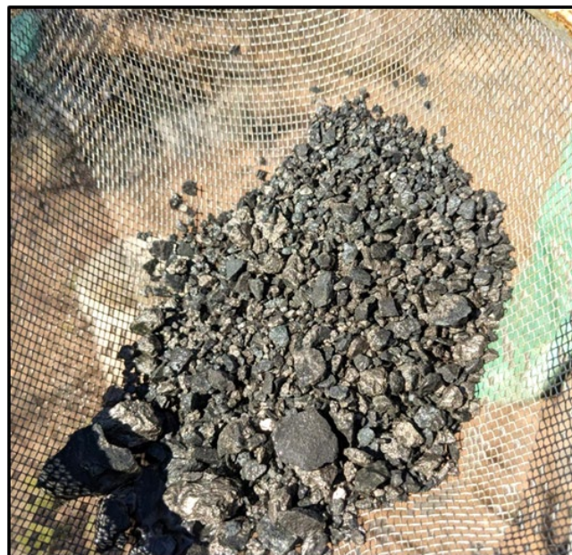
Figure 6 – Disseminated and matrix sulphides in RC drill chips (53m in NRC455)
